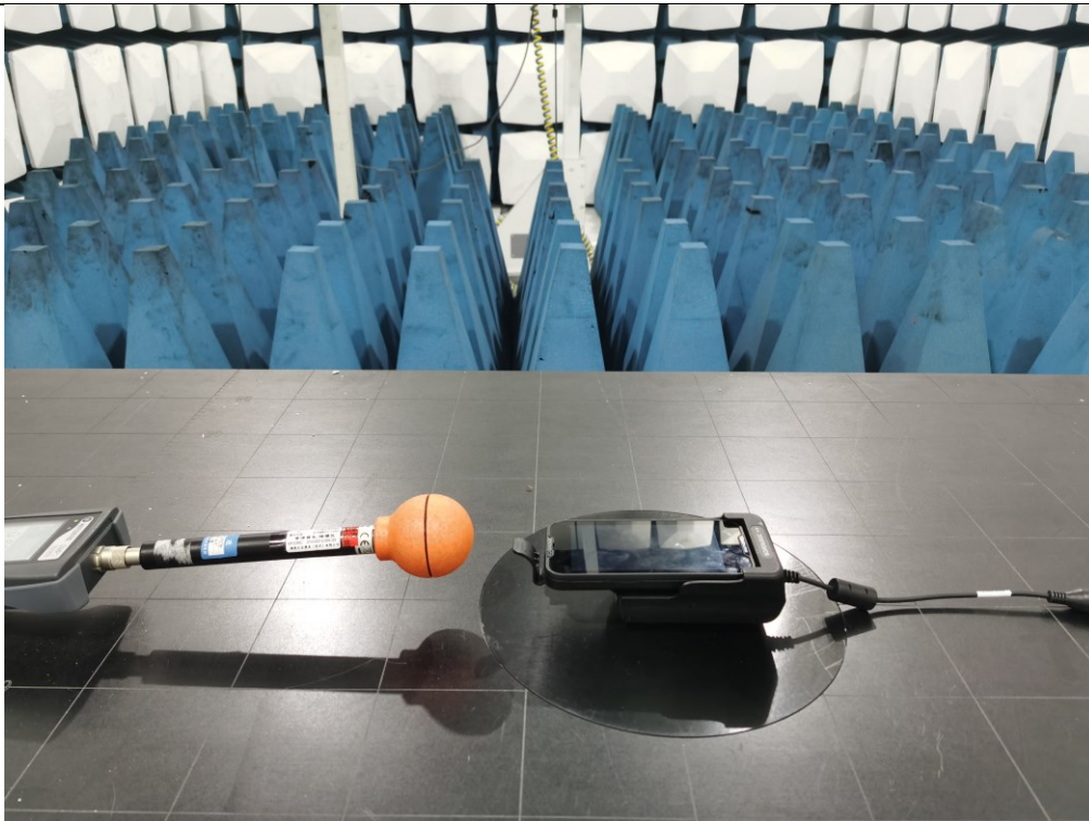
Description: RF Exposure Setup –Above 100kHz
