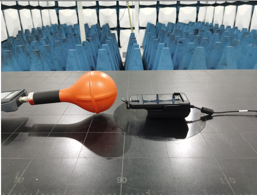
Description: RF Exposure Setup –Above 100kHz
