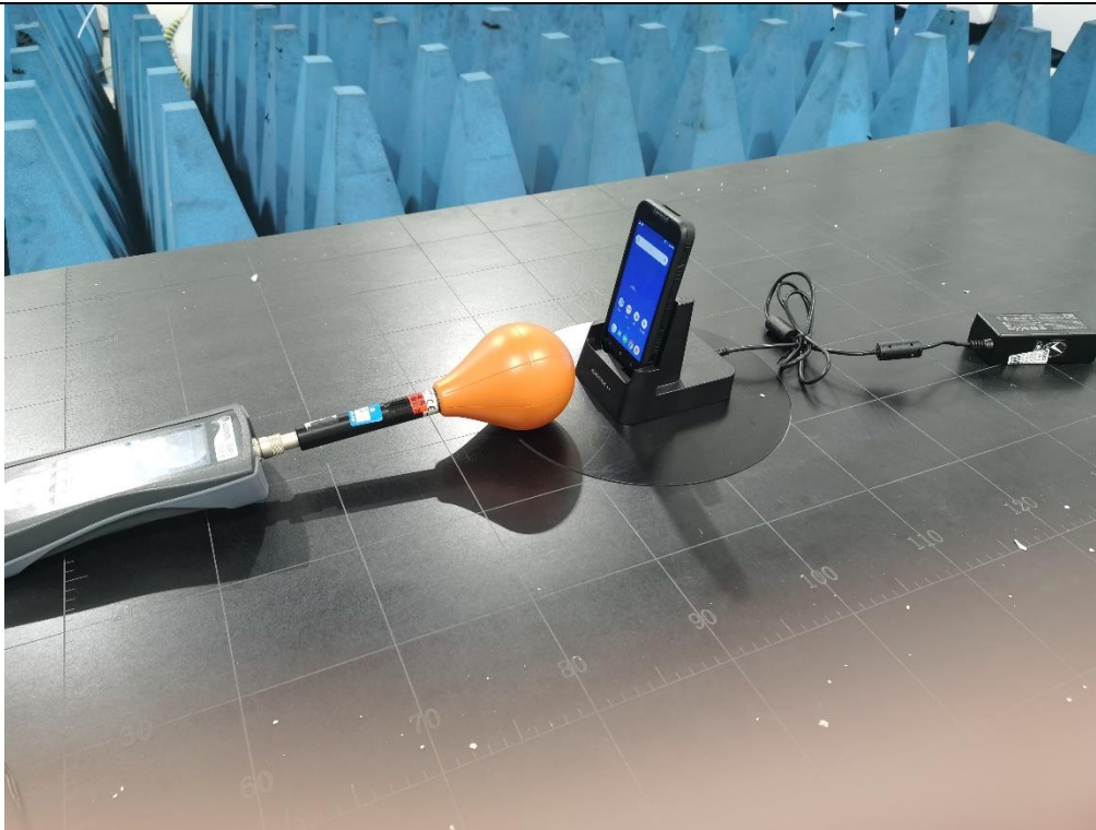
Description: RF Exposure Setup –Above 100kHz
