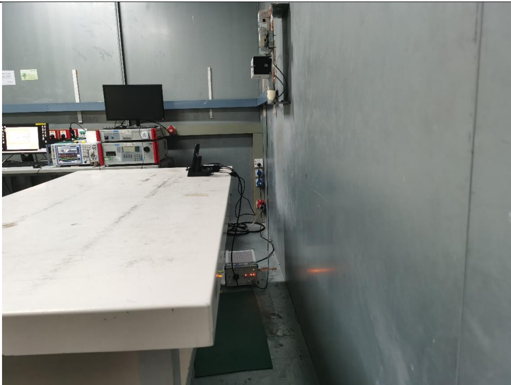
Description: AC Power Line Conducted Emission
