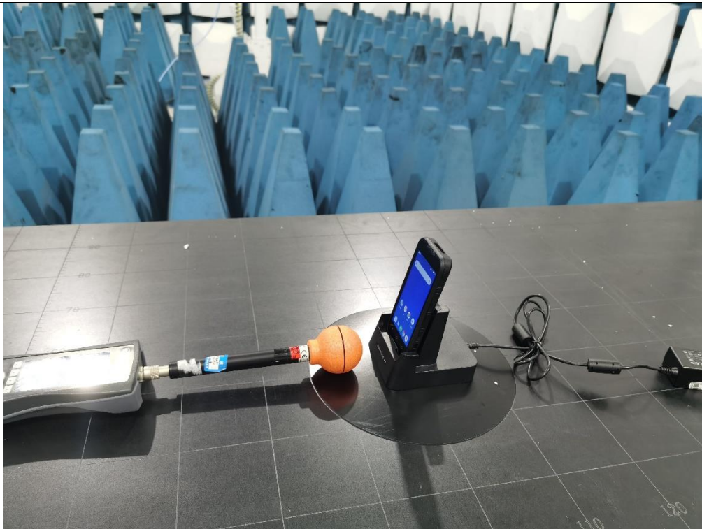
Description: RF Exposure Setup –Above 100kHz
