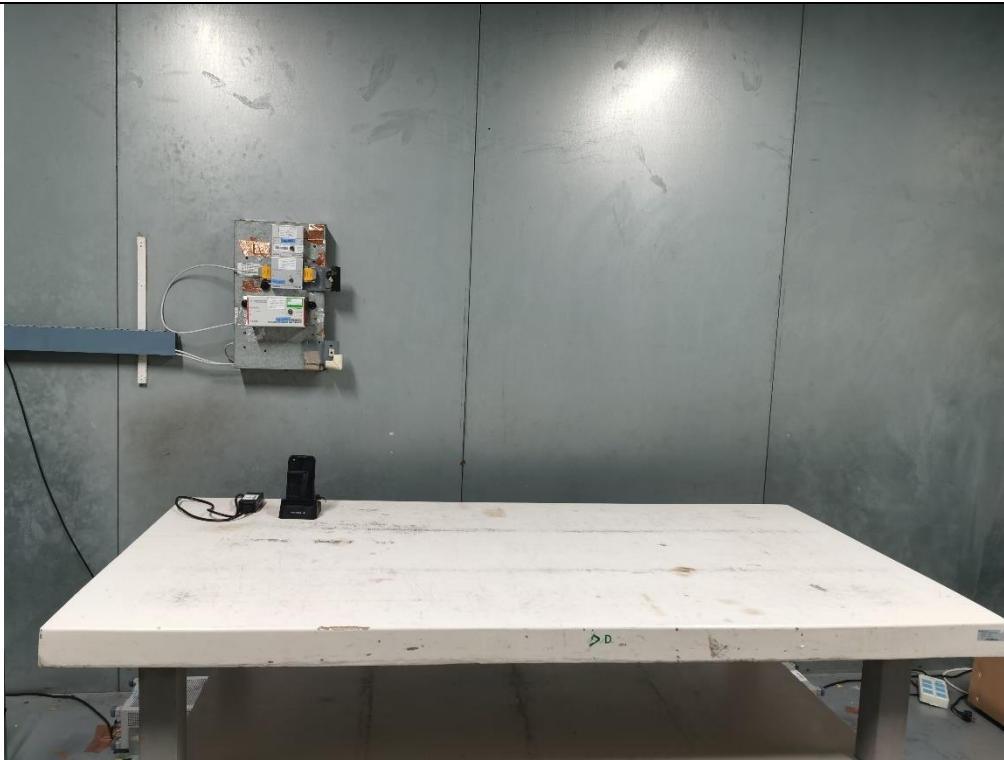
Description: AC Power Line Conducted Emission
