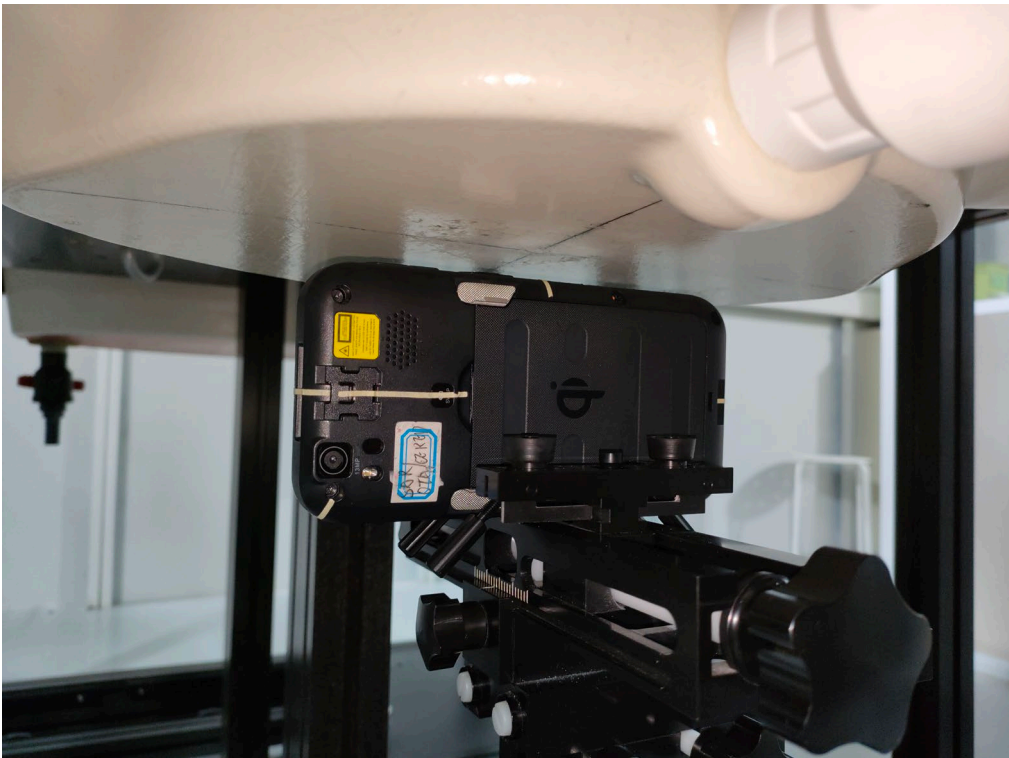
Description: Body Right Position with 10mm gap
