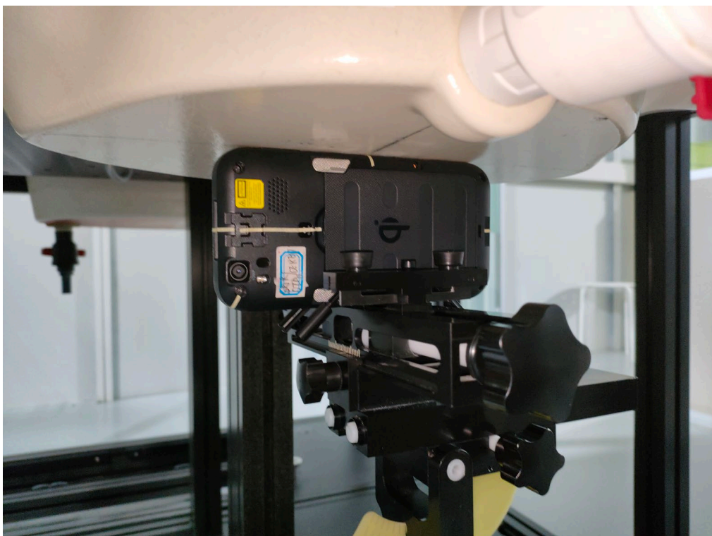
Description: Extremity Right Position with 0mm gap
