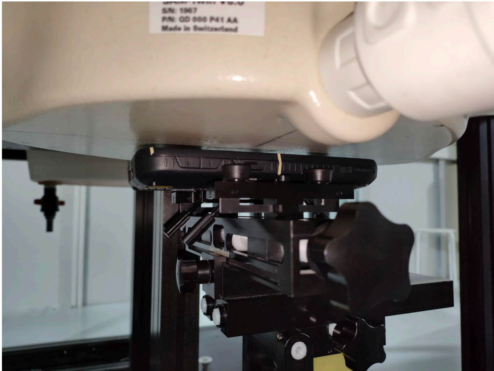
Description: Body Back Position with 10mm gap
