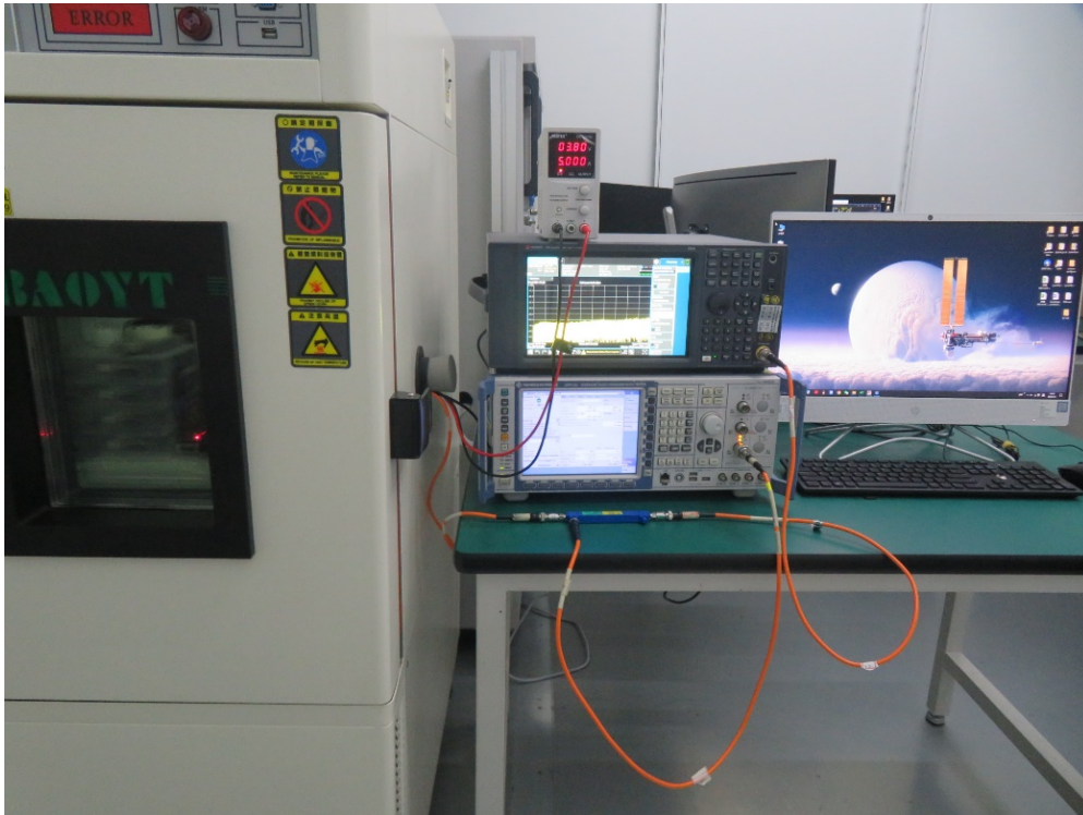
Description: DFS Test Setup
