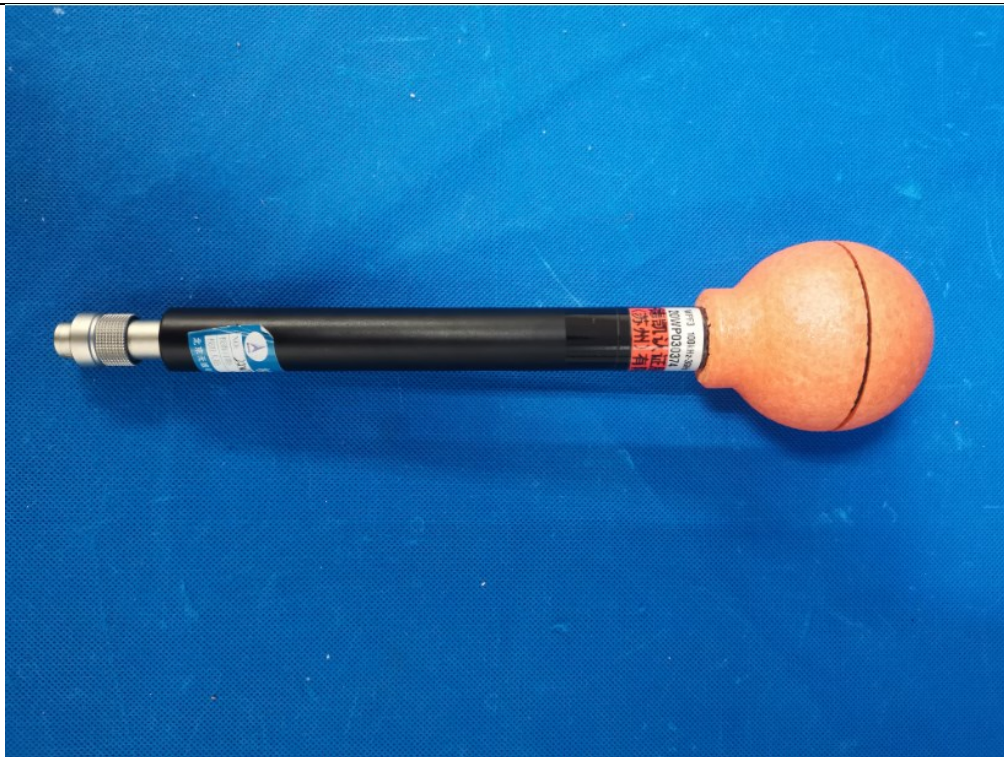
Description: RF Exposure Setup –Test Probe 100kHz ~ 3GHz
