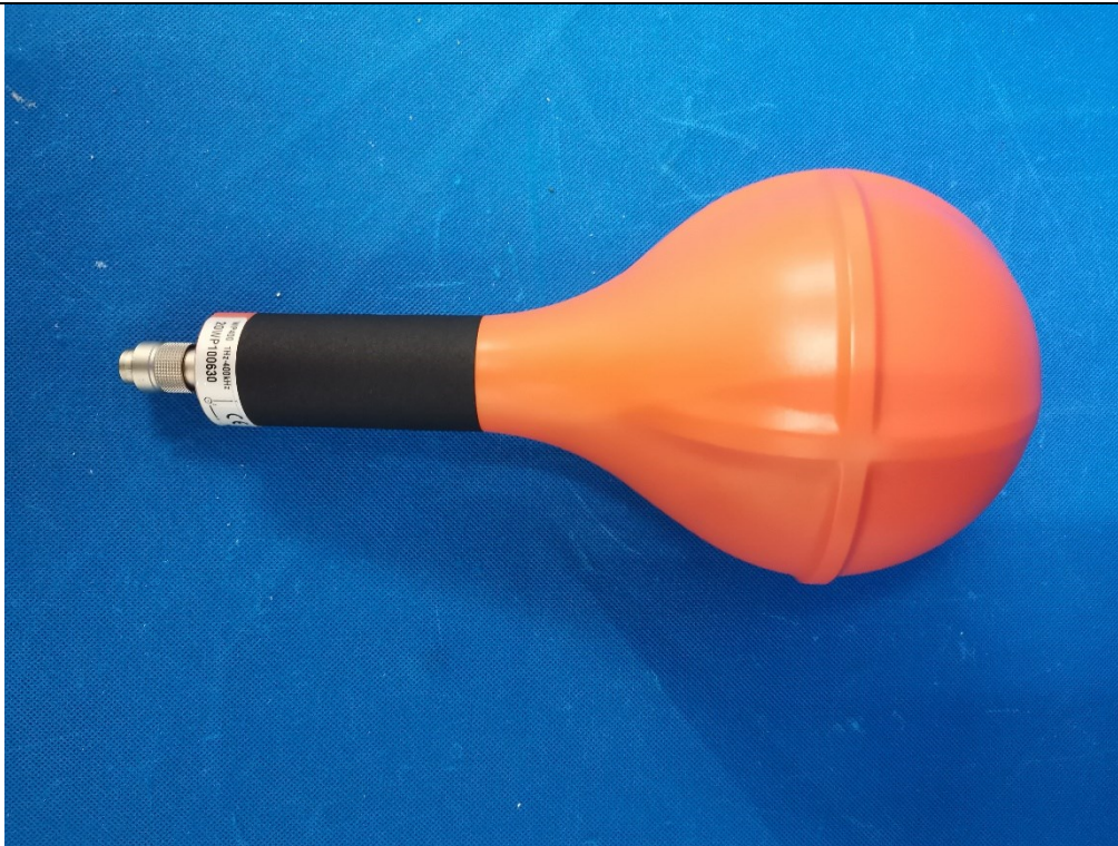
Description: RF Exposure Setup –Test Probe 100kHz ~ 3GHz
