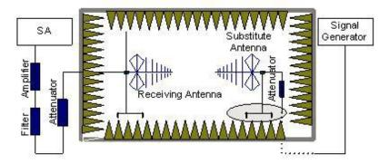
In the chamber, an substitution antenna for the frequency band of interest is placed at the reference point of the chamber. An RF Signal source for the frequency band of interest is connected to the substitution antenna with a cable that has been constructed to not interfere with the radiation pattern of the antenna. A power (P<sub>Mea</sub>) is applied to the input of the
