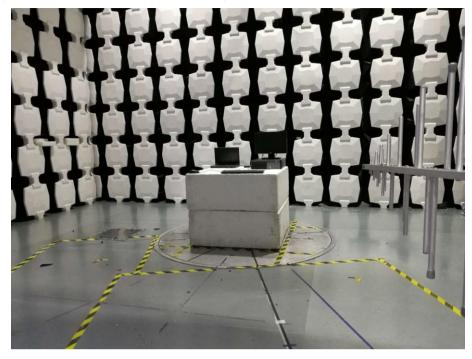
Description: Radiated Emission Test Setup
