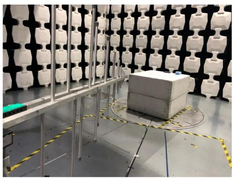
Description: Radiated Emission Test Setup
