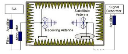
In the chamber, an substitution antenna for the frequency band of interest is placed at the reference point
