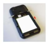
4. Replace the battery (see **Battery Installation**).
