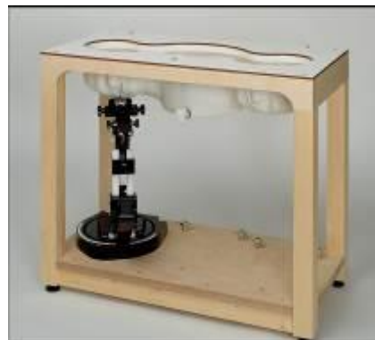
Picture C.9: SAM Twin Phantom
