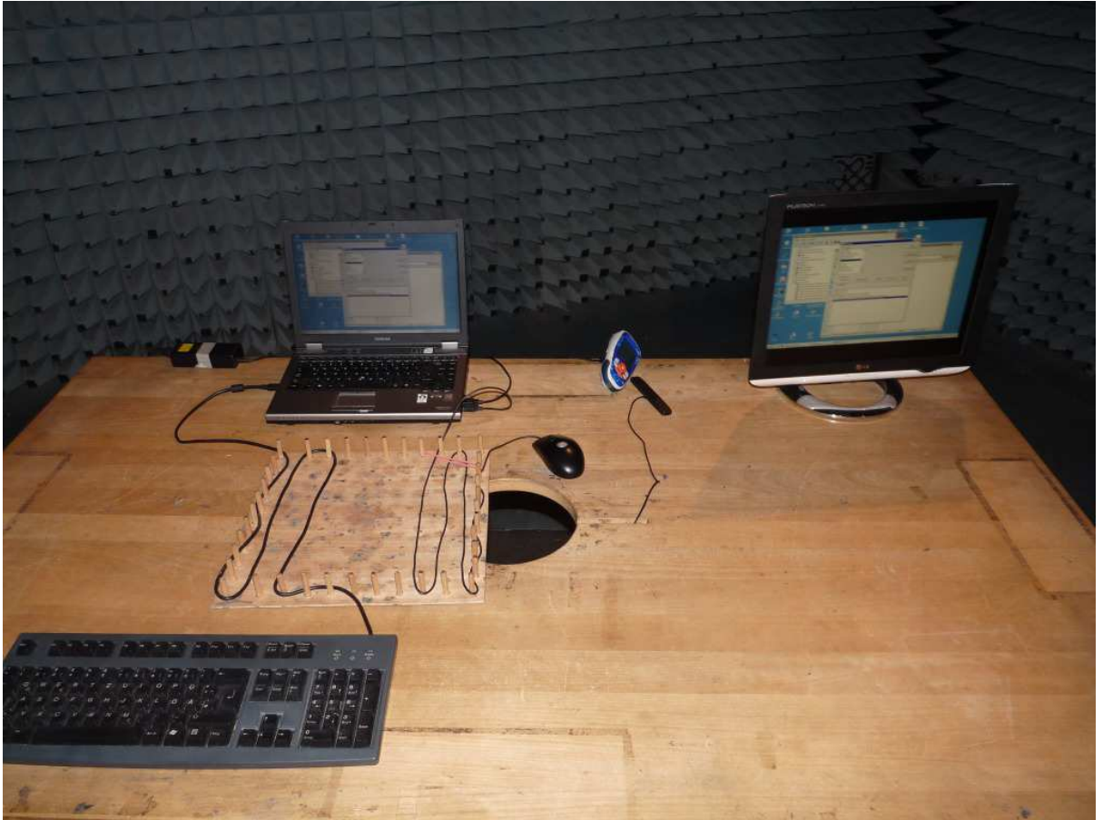
Test Setup (radiated measurement) Computer peripheral setup
