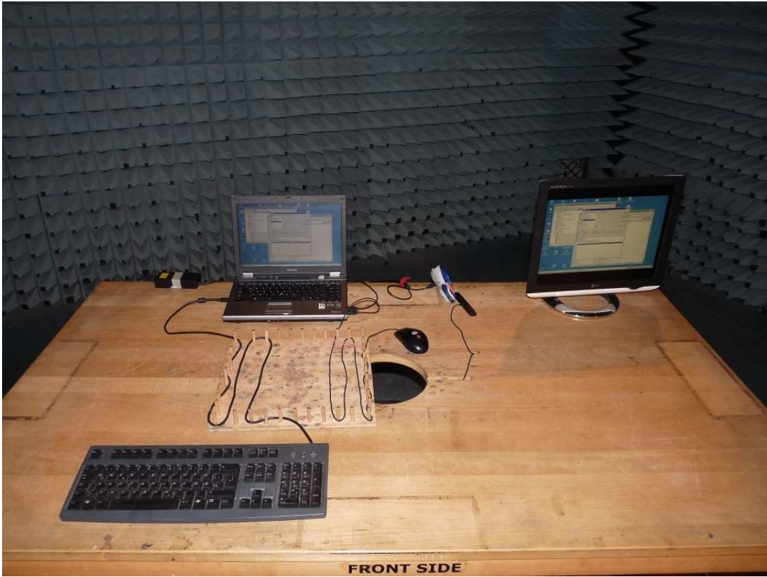
Photo 3: Test setup for radiated measurements (Enclosure, 30 MHz to 1 GHz)
