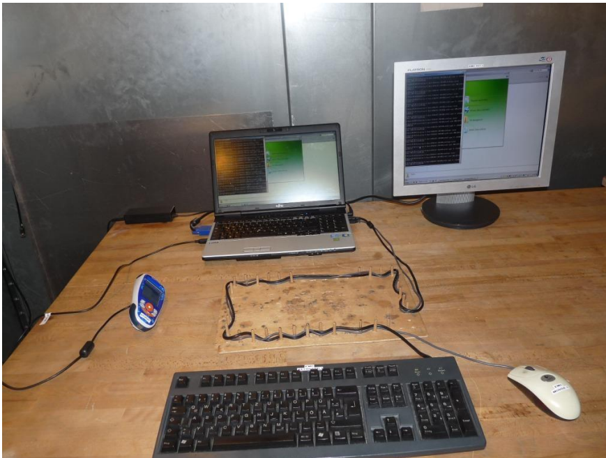
Photo 1: Test setup for conducted measurements (computer peripheral setup, EUT connected via USB cable to computer, intentional/ unintentional radiator §15.)
