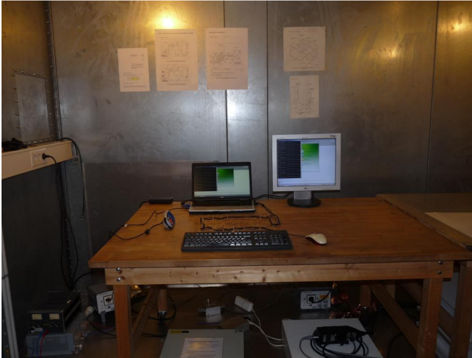
Photo 1: Test setup for conducted measurements (computer peripheral setup, EUT connected via USB cable to computer, intentional/ unintentional radiator §15.)
