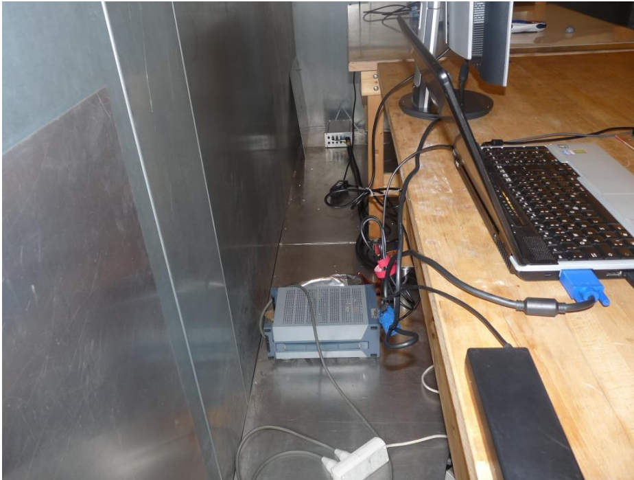
Photo 3: Test setup for conducted measurements (computer peripheral setup, EUT connected via USB cable to computer, intentional/ unintentional radiator §15.)
