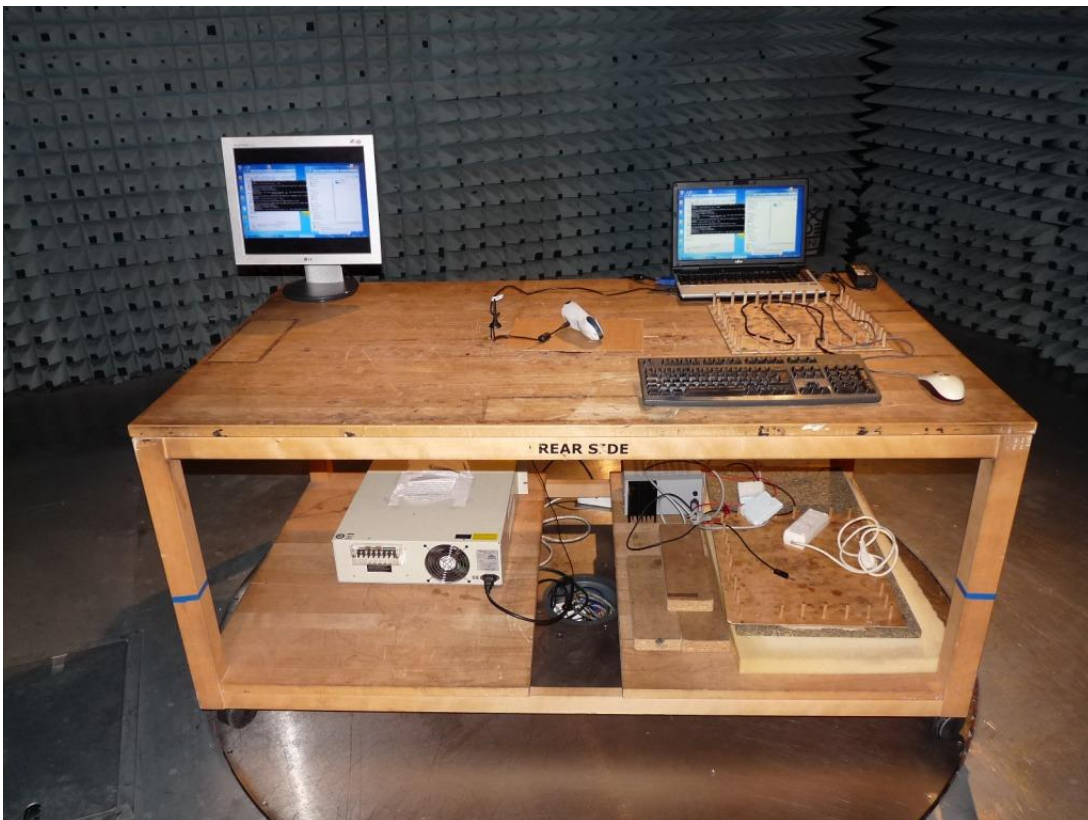
Photo 4: Test setup for radiated measurements, computer peripheral setup, EUT connected via USB cable to computer, intentional/ unintentional radiator §15.
