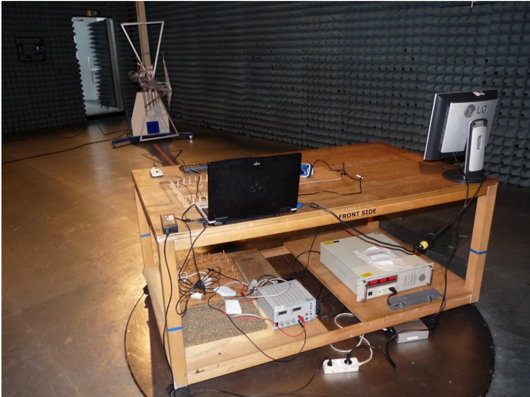
Photo 5: Test setup for radiated measurements, computer peripheral setup, EUT connected via USB cable to computer, intentional/ unintentional radiator §15.
