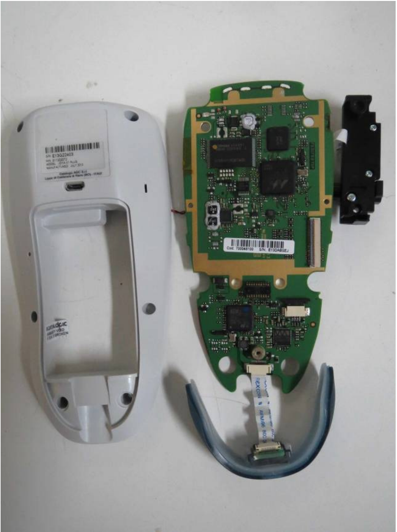
MAIN BOARD FRONT VIEW
