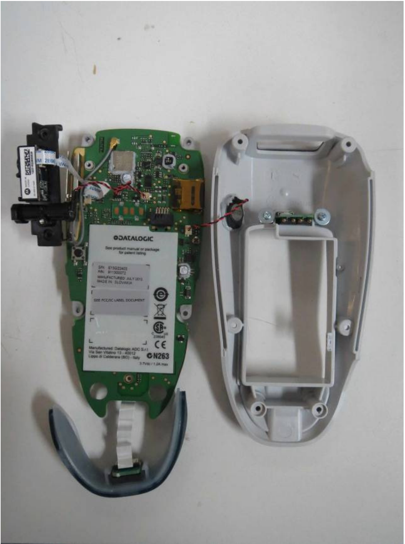
MAIN BOARD REAR VIEW
