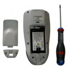
2. Remove the cover and then the battery pack, using the proper plastic strips. Pay attention when disconnecting the connector.
