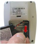
Install the new battery pack, first insert the connector respecting the right way, then the upper side, finally the bottom side, leaving the plastic strip available for future replace.
