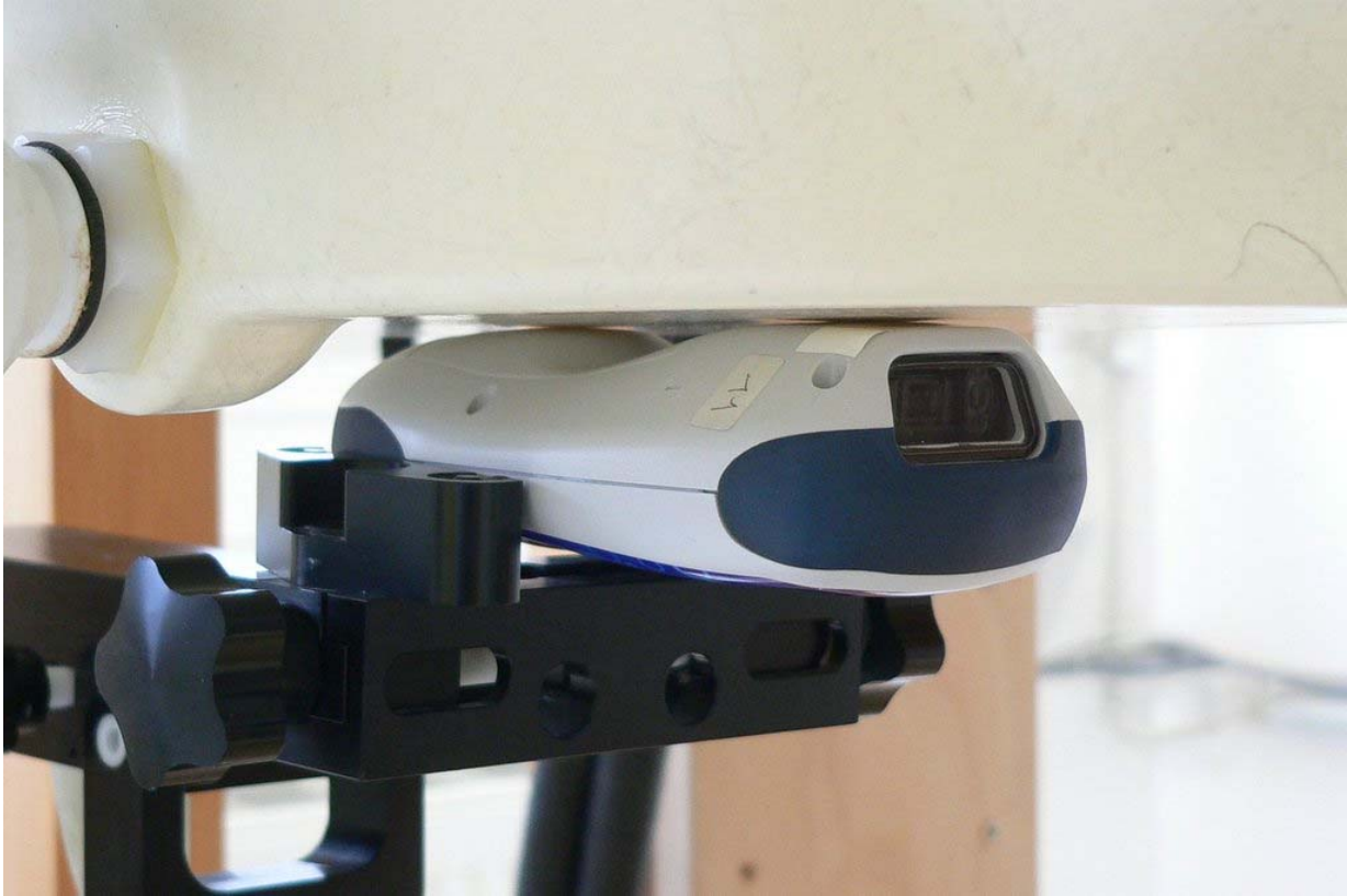
Fig. 12: Body worn configuration for Joya X1 Plus, position 1, display towards the ground, 0 mm distance.
