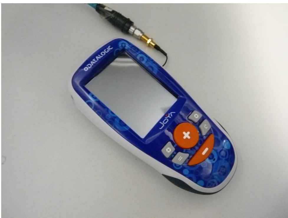
Photo 4: Test setup for conducted measurements
