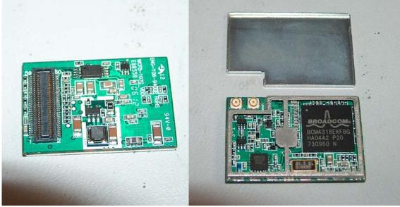
The SDC-MCF10G is designed specifically for integration in small form factor application specific devices and the challenging RF environments in which they operate. Shown here clockwise from the top is the antenna connector side of the device, the same side wit the shield removed and the host connector side.
