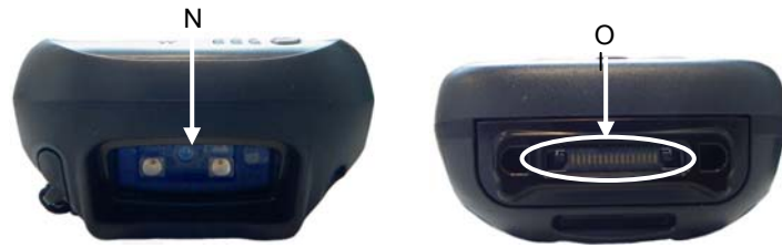
N) Data Capture/Laser Output Window O) HandyLink™ Connector (host/device)
