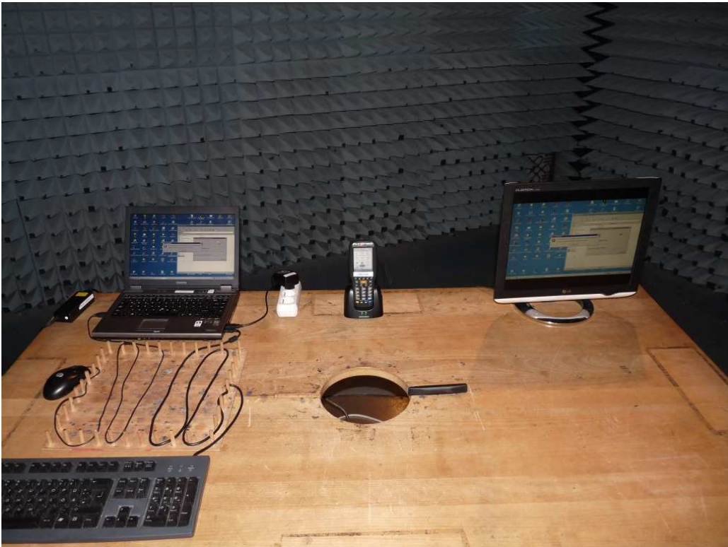
Photo 6: Test setup for radiated measurements (30 MHz to 1 GHz) (Single Slot Dock / RS232+USB connection to PC / Ext.Battery)
