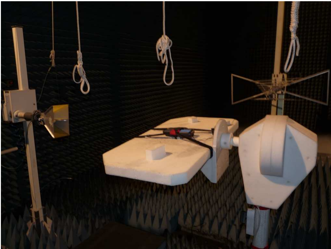
Photo 3: Test setup for radiated measurements (above 1 GHz)
