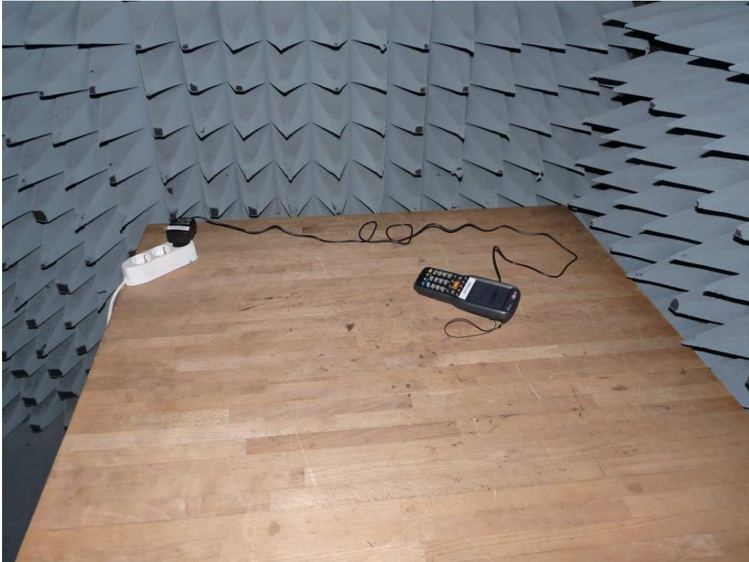
Photo 1: Test setup for radiated measurements (below 30 MHz)
