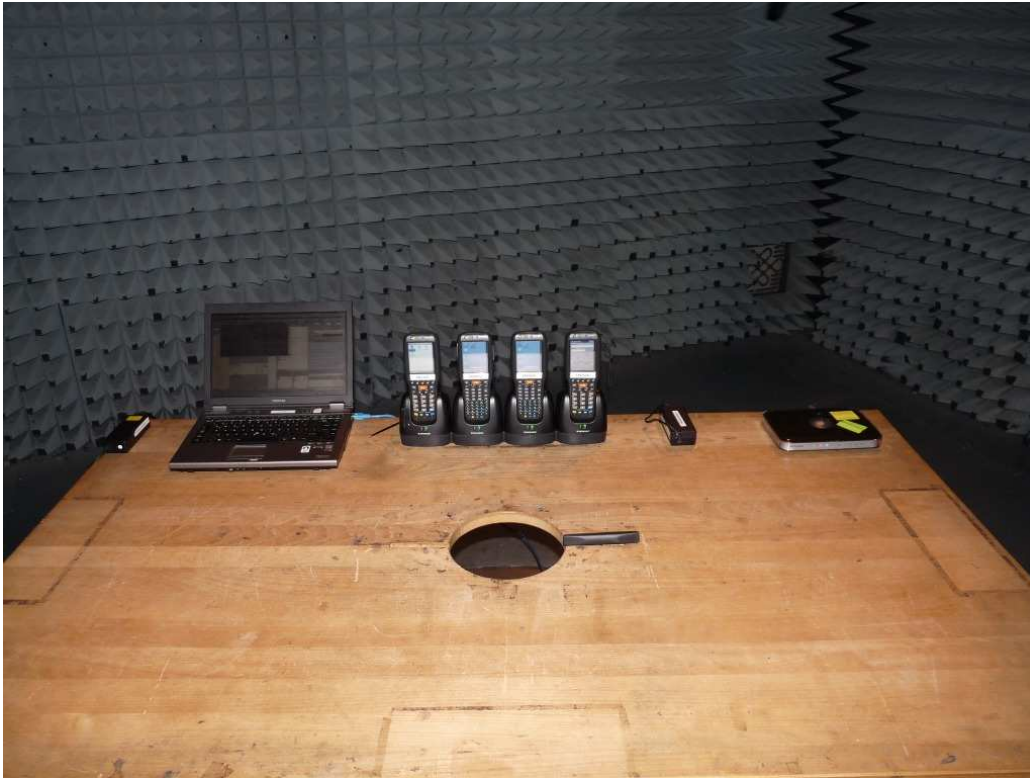
Photo 7: Test setup for radiated measurements (30 MHz to 1 GHz) (MultiSlotDock(4Units)/LAN con.to PC(via Router)/Ext.&Std.Bat)
