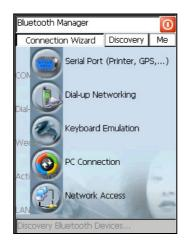
3. Tap on the "Me" button to enter the related window; then, tap on the "ON" button to activate the Bluetooth<sup>®</sup> module. The module activation may be also performed by using the WIRELESS COMMUNICATION applet as described in par. 3.8.4.
