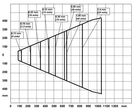
Guaranteed Reading Diagram at 47° - Reading Zones (10° skew angle)
