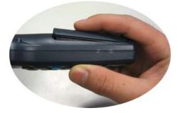
5. Press it until the battery latch is automatically closed.
