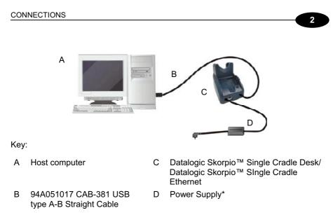
\* Recommended Power Supply: FPS18 AC/DC Power Supply (94ACC4595).
