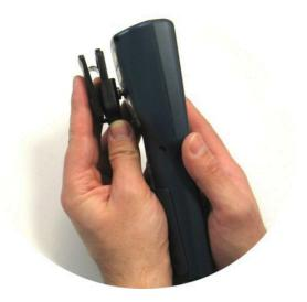
4. To release the terminal, press the belt clip unlock button.
