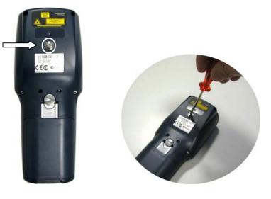
2. Screw the belt clip pivot on the terminal by using the fixing screw.
