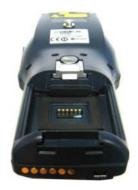
1b. Turn off the Datalogic Skorpio-GUN<sup>™</sup> and remove the battery pack, by pulling the battery latch down.
