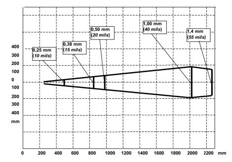
Guaranteed Reading Diagram - Reading Zones (10° skew angle)
