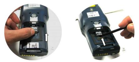
To remove the Mini SD card, just push it toward the inside, aided by the stylus, until it clicks; a spring system will return it out.
