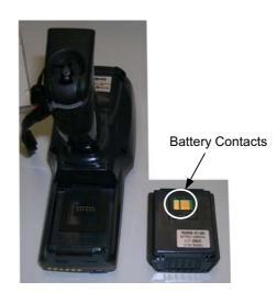
3. To correctly insert the new battery pack, first insert the bottom and then the upper part of the battery pack into the slot as indicated in the following figure:
