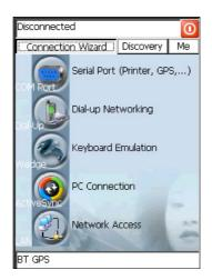
The "Serial Port" button starts communication through the Bluetooth  $^{\ensuremath{\mathbb{B}}}$  serial port COM 5.
