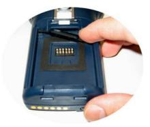
3. Insert the card with the written part upward (as shown in the figure) and push it in, aided by the stylus, until it clicks into place.
