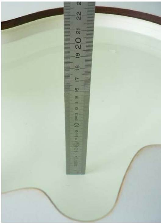
Fig. 27: Liquid depth for IEEE 802.11 b/g Head measurements
