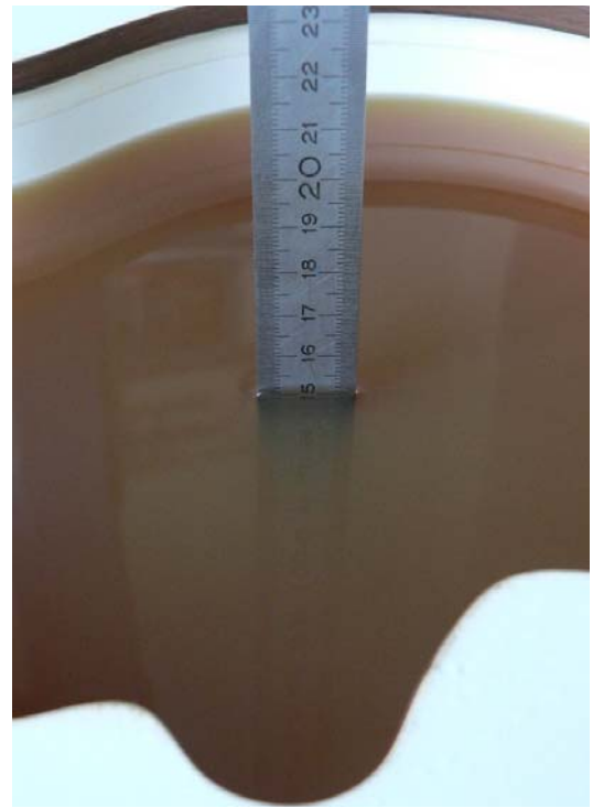
Fig. 28: Liquid depth for IEEE 802.11 a Head measurements
