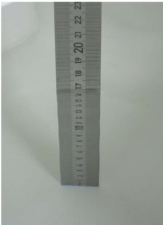
Fig. 29: Liquid depth for IEEE 802.11 b/g Body measurements
