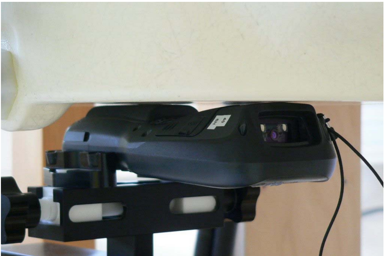
Fig. 29: Body worn configuration, position 2, display towards the ground.
