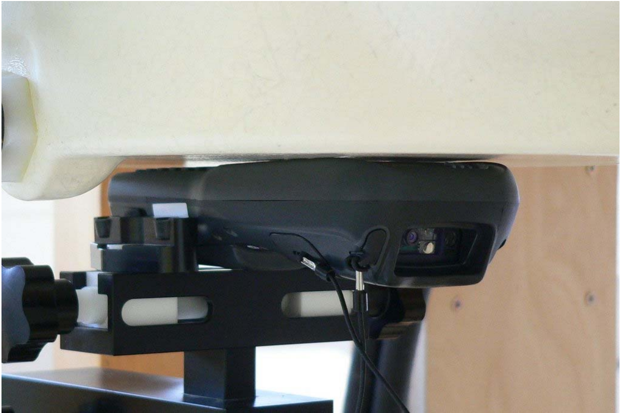
Fig. 28: Body worn configuration, position 1, display towards the phantom.
