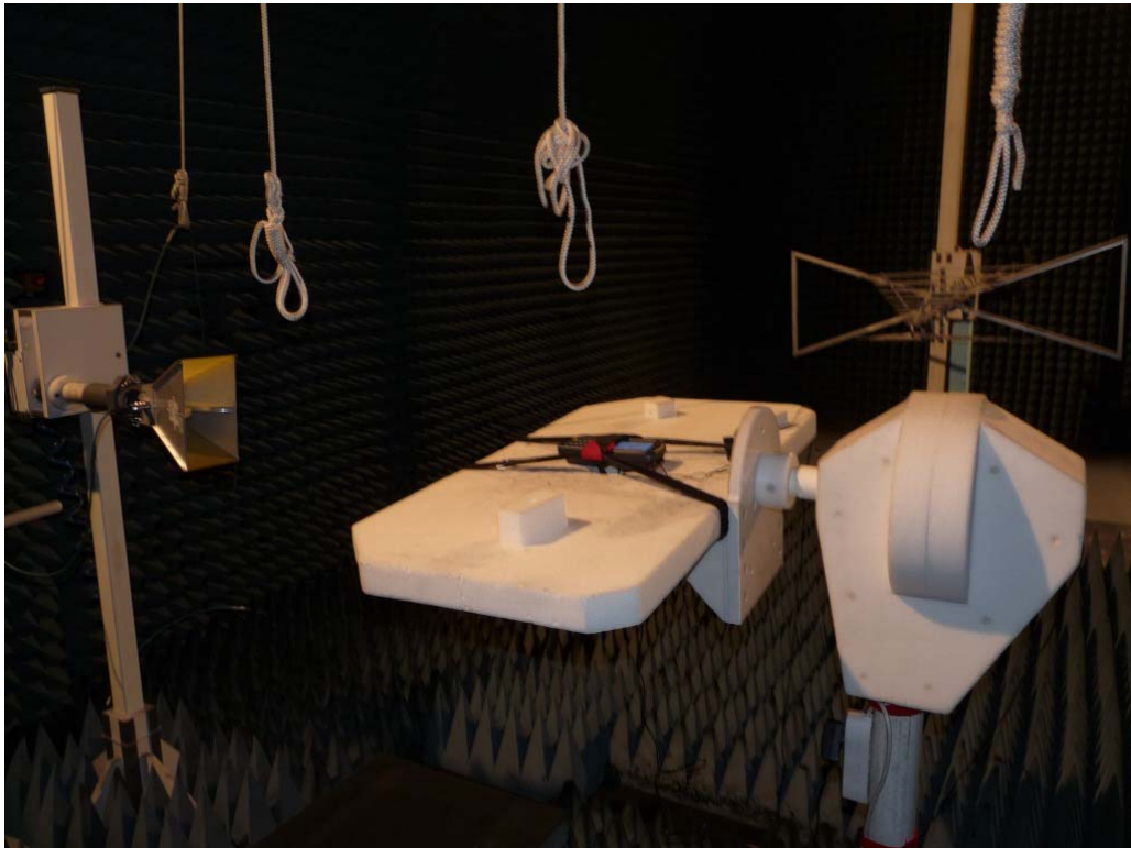
Photo 3: Test setup for radiated measurements (above 1 GHz)
