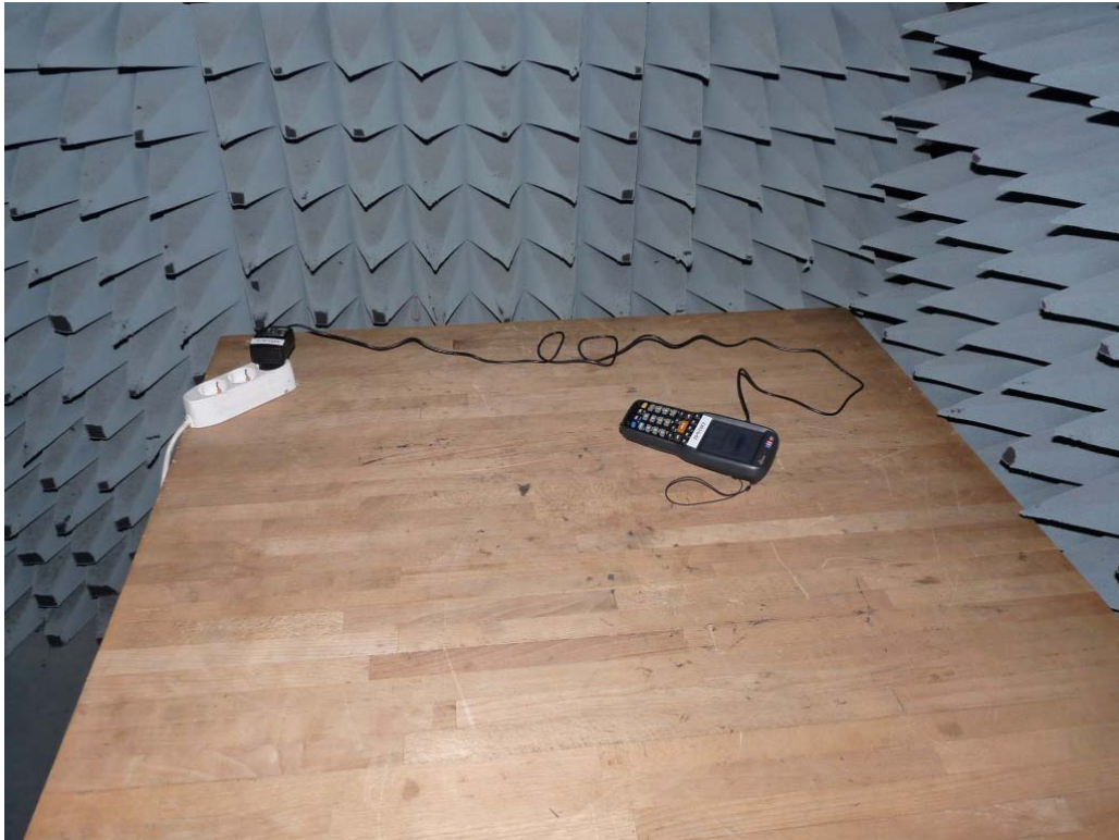
Photo 1: Test setup for radiated measurements (below 30 MHz)
