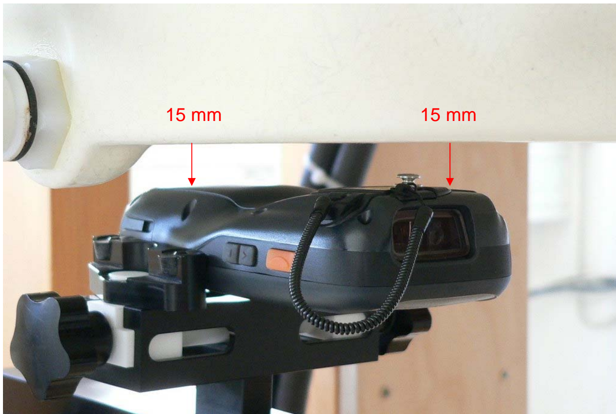
Fig. 17: Body worn configuration, display towards the ground, 15 mm distance.
