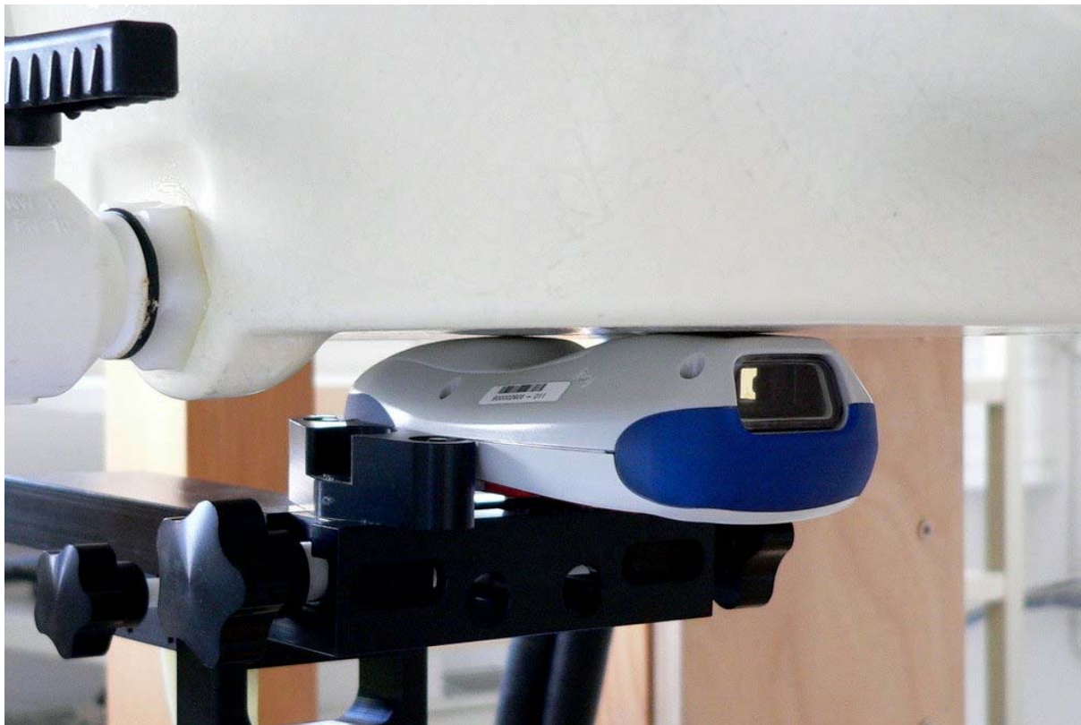
Fig. 17: Body worn configuration with the back of the device in direct contact against the flat phantom, display towards the ground
