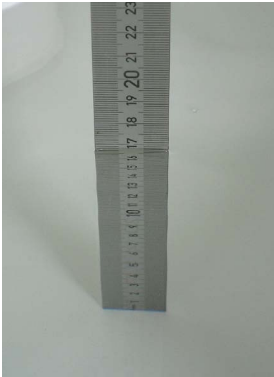
Fig. 19: Liquid depth for IEEE 802.11 b/g Body measurements
