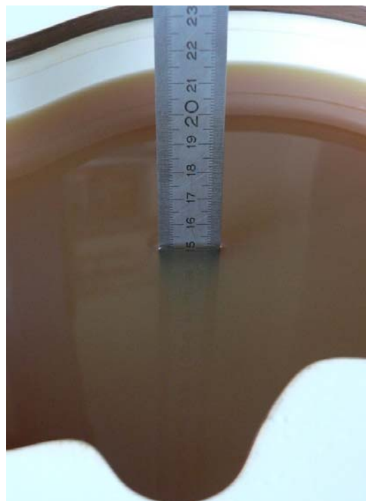
Fig. 67: Liquid depth for IEEE 802.11 a Head measurements
