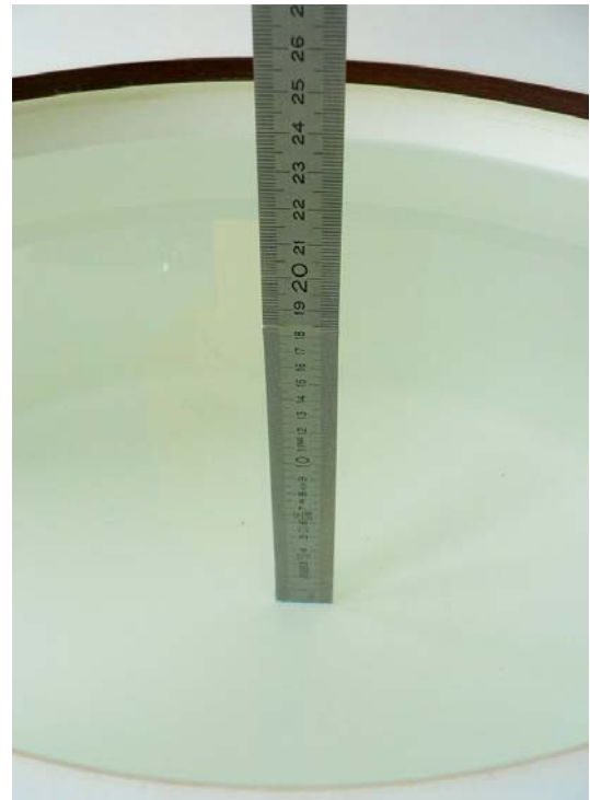
Fig. 69: Liquid depth for PCS 1900 and WCDMA II Body measurements
