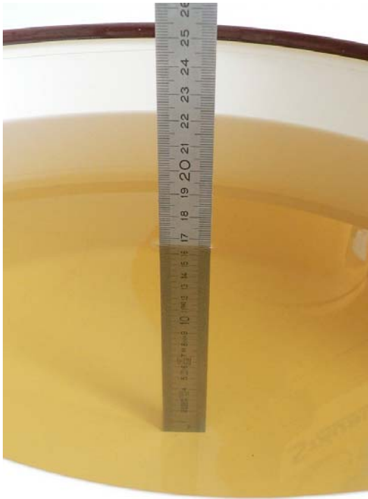
Fig. 68: Liquid depth for GSM 850 and WCDMA V Body measurements
