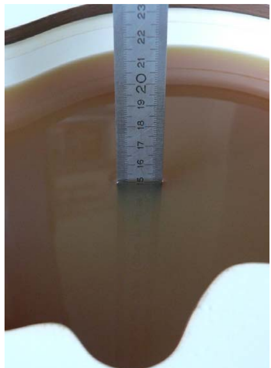
Fig. 67: Liquid depth for IEEE 802.11 a Head measurements
