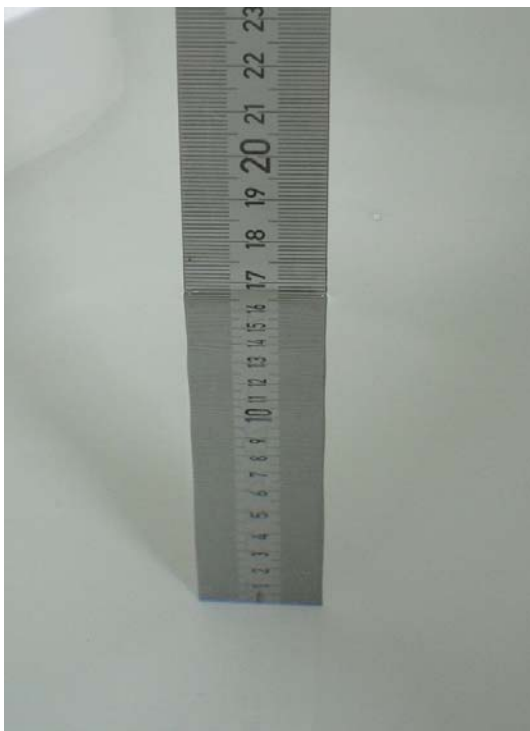
Fig. 70: Liquid depth for IEEE 802.11 b/g Body measurements
