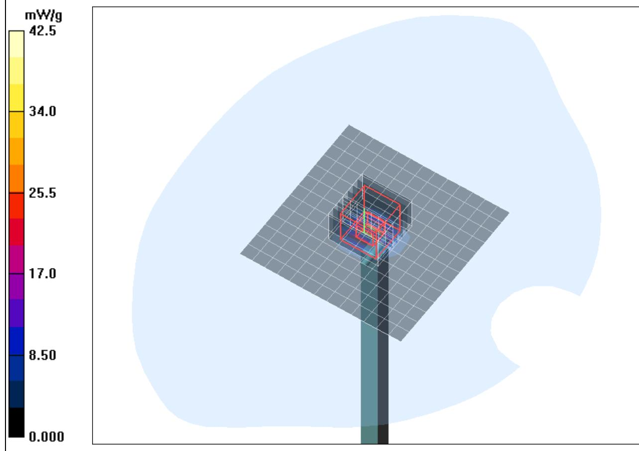
**SAR result with Body TSL at 5800 MHz****Test Laboratory: IMST GmbH, DASY Blue (I); File Name: [260410\\_b\\_3536\\_5800.da4](#)****DUT: Dipole 5GHz SN: 1028; Type: D5GHzV2; Serial: D5GHzV2 - SN:1028****Program Name: System Performance Check at 5800 MHz**
