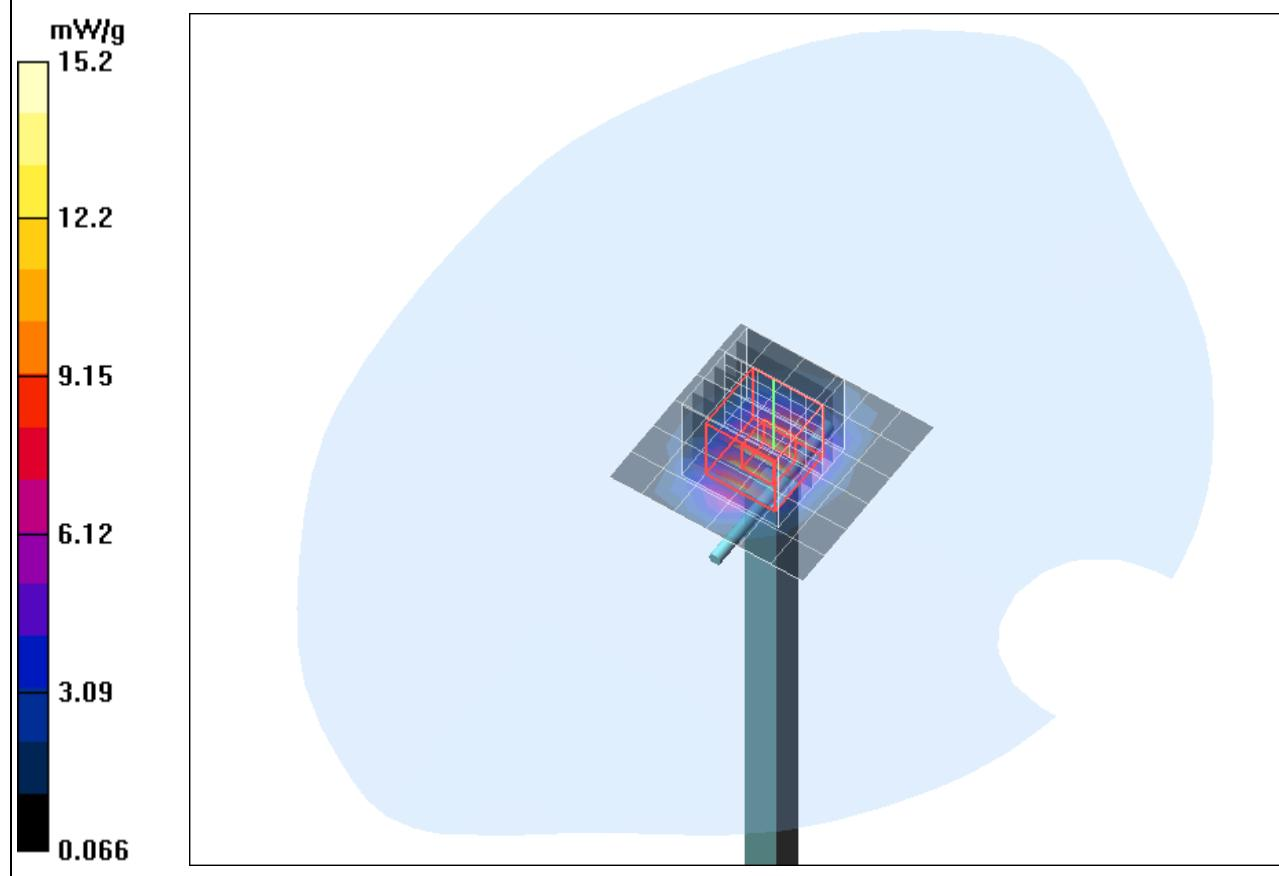
**SAR result with Body TSL****Test Laboratory: Imst GmbH, DASY Yellow (II); File Name: [081209\\_y\\_3536.da4](#)****DUT: Dipole 2450 MHz SN: 709; Type: D2450V2; Serial: D2450V2 - SN:709****Program Name: System Performance Check at 2450 MHz**
