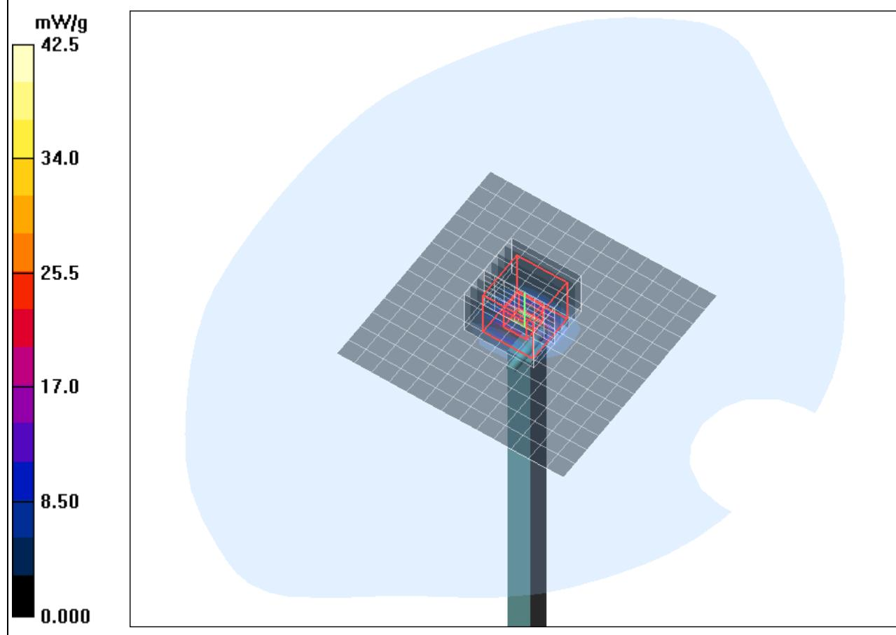
**SAR result with Head TSL at 5800 MHz****Test Laboratory: IMST GmbH, DASY Blue (I); File Name: [270410\\_b\\_3536\\_5800.da4](#)****DUT: Dipole 5GHz SN: 1028; Type: D5GHzV2; Serial: D5GHzV2 - SN:1028****Program Name: System Performance Check at 5800 MHz**
