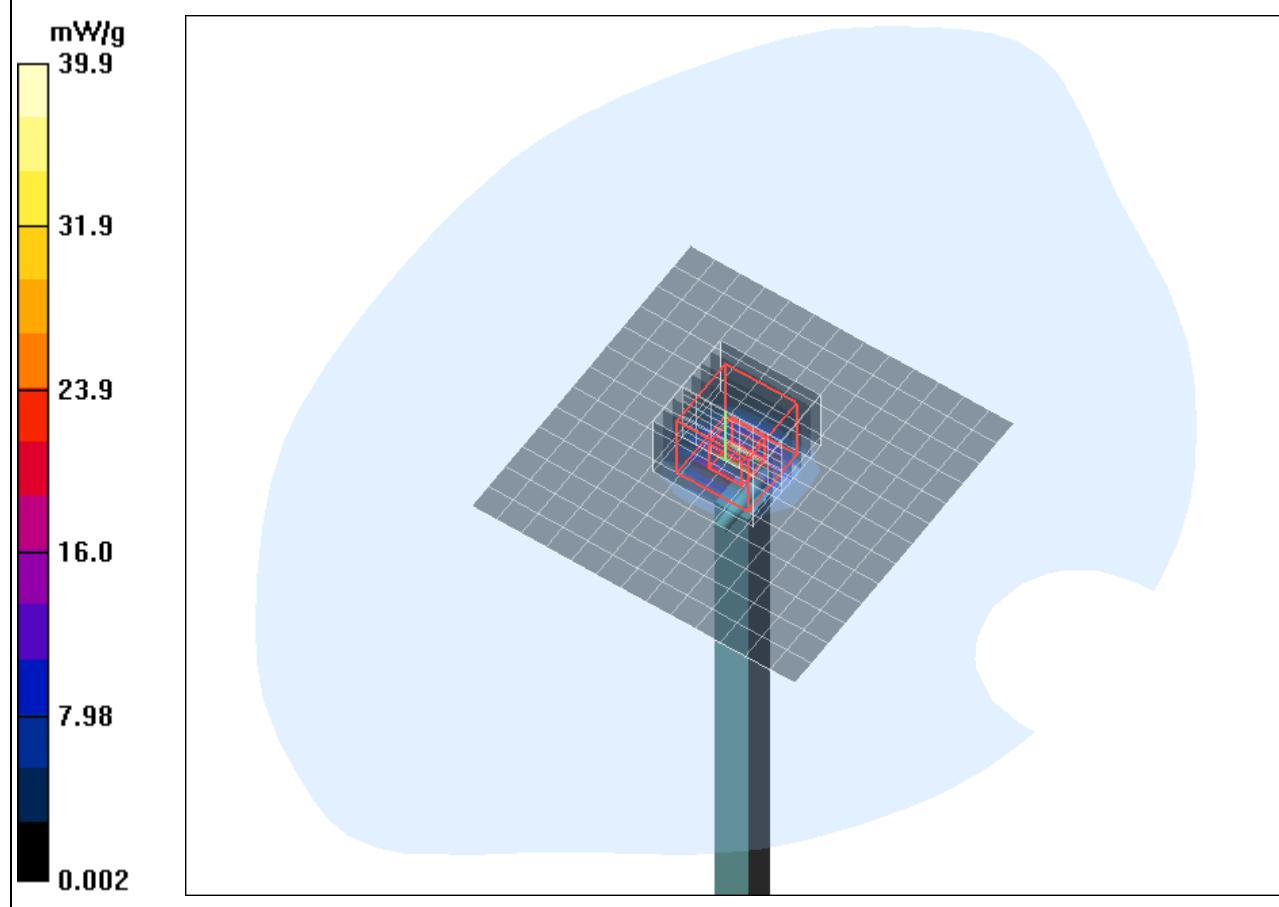
**SAR result with Head TSL at 5500 MHz****Test Laboratory: IMST GmbH, DASY Blue (I); File Name: [270410\\_b\\_3536\\_5500.da4](#)****DUT: Dipole 5GHz SN: 1028; Type: D5GHzV2; Serial: D5GHzV2 - SN:1028****Program Name: System Performance Check at 5500 MHz**
