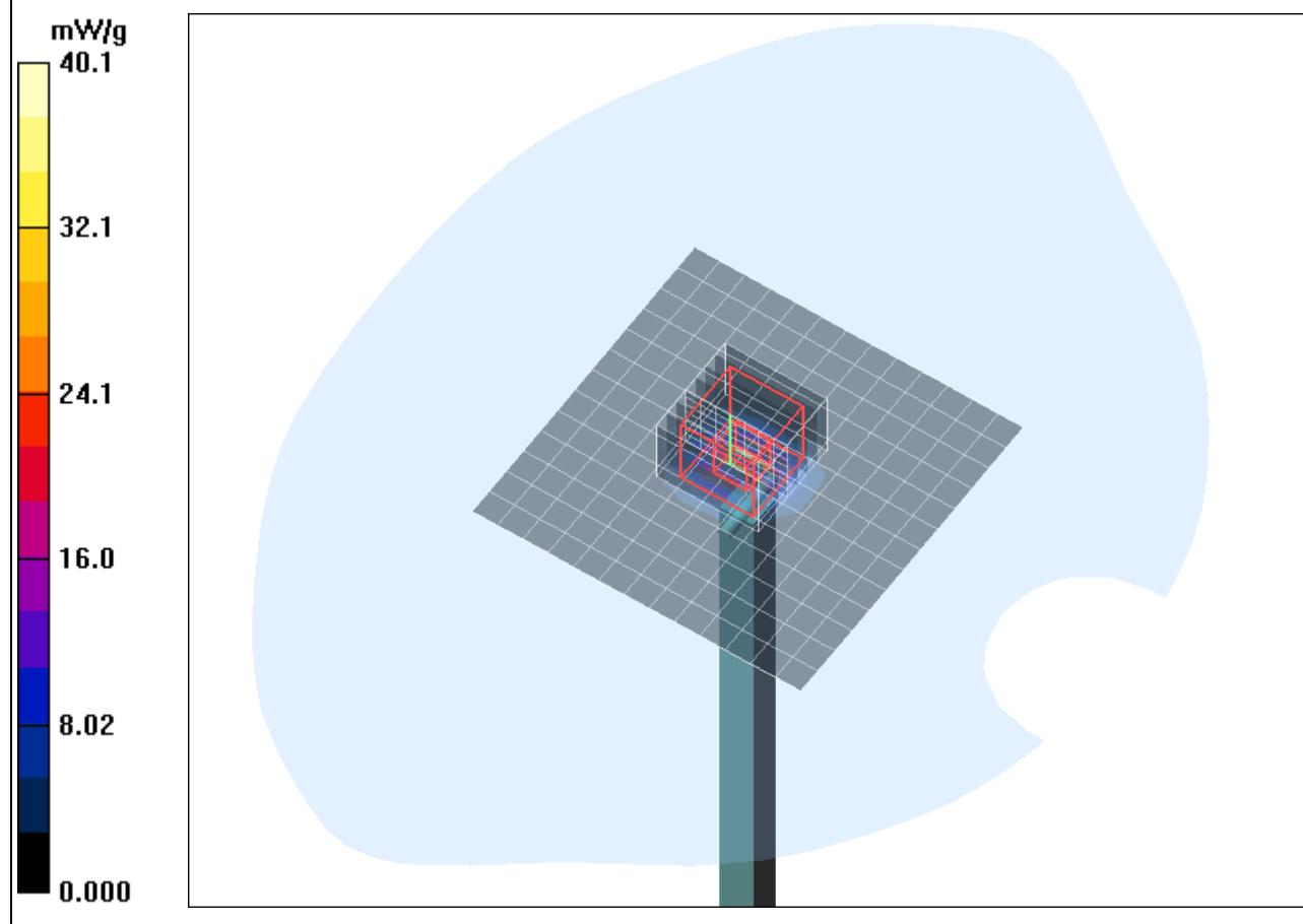
**SAR result with Body TSL at 5200 MHz****Test Laboratory: IMST GmbH, DASY Blue (I); File Name: [260410\\_b\\_3536\\_5200.da4](#)****DUT: Dipole 5GHz SN: 1028; Type: D5GHzV2; Serial: D5GHzV2 - SN:1028****Program Name: System Performance Check at 5200 MHz**
