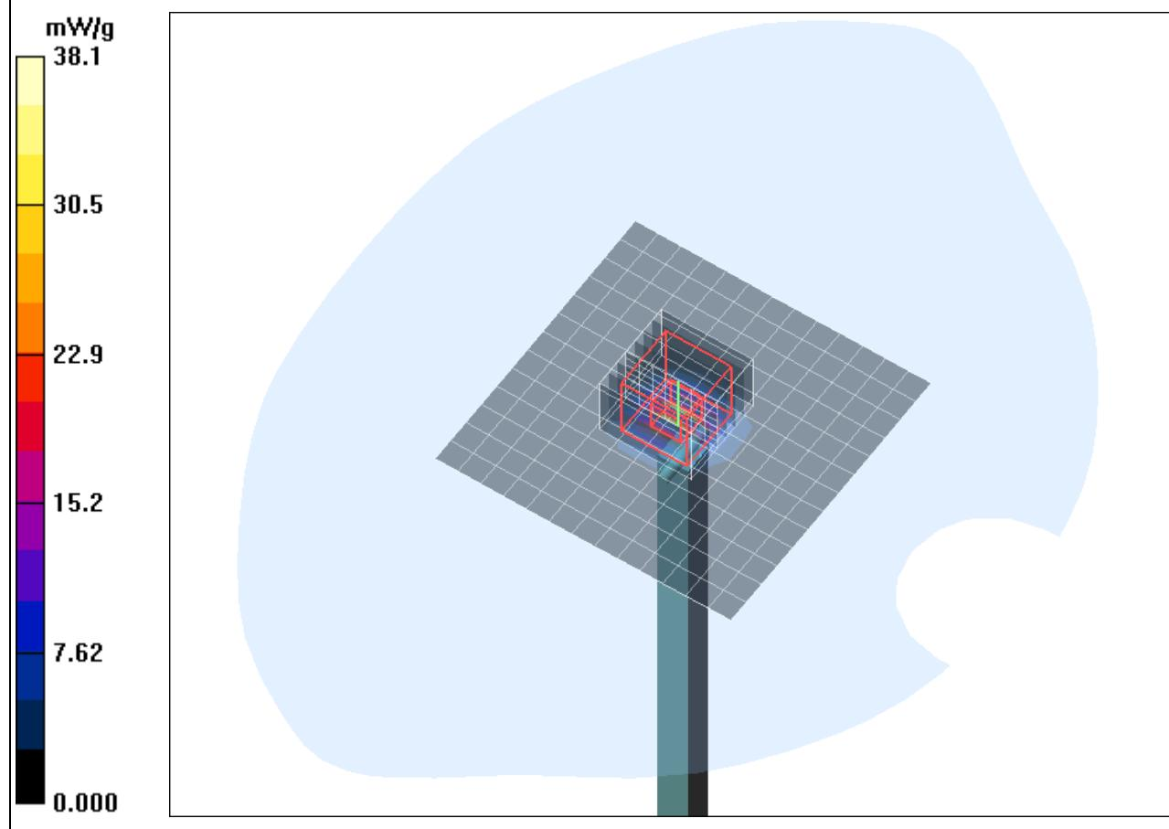
**SAR result with Body TSL at 5500 MHz****Test Laboratory: IMST GmbH, DASY Blue (I); File Name: [260410\\_b\\_3536\\_5500.da4](#)****DUT: Dipole 5GHz SN: 1028; Type: D5GHzV2; Serial: D5GHzV2 - SN:1028****Program Name: System Performance Check at 5500 MHz**
