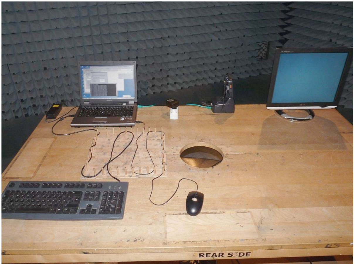
setup for radiated tests, EUT + Cradle + AC/DC adapter (of cradle); LAN connection to Laptop
