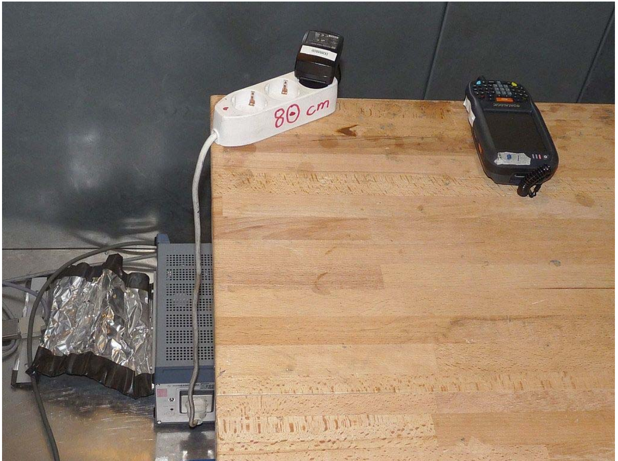
setup for conducted tests, EUT + AC/DC adapter
