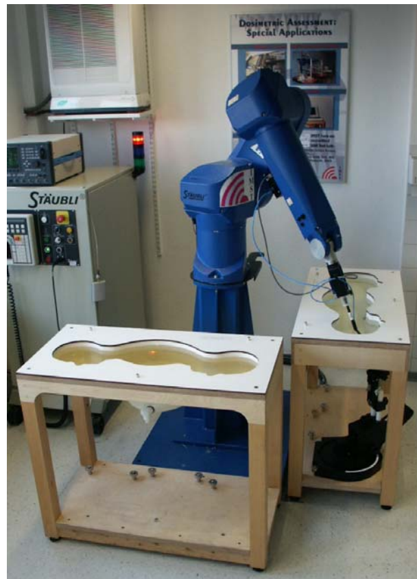
Fig. 8: The measurement set-up with two SAM phantoms containing tissue simulating liquid.
