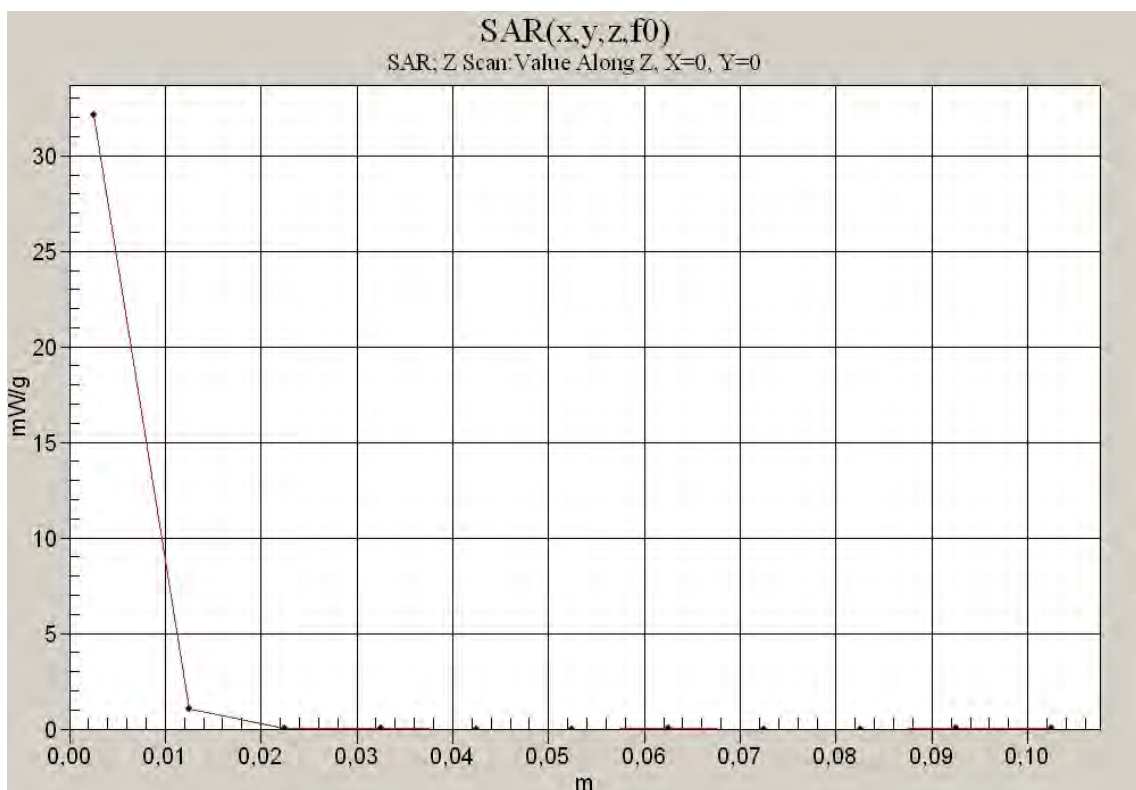
Fig. 106: SAR versus liquid depth, 5800 MHz, body (May 14, 2010; Ambient Temperature: 21.8° C; Liquid Temperature: 21.2° C).
