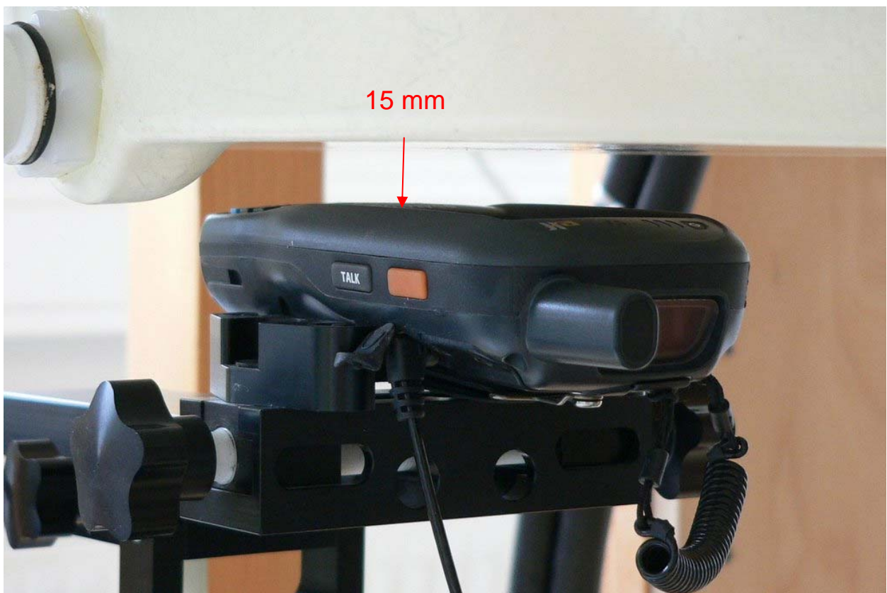
Fig. 53: Top view of body worn, HS connected, display up (towards the phantom).
