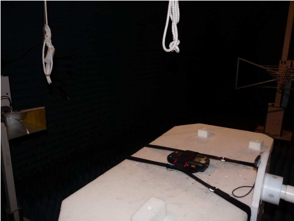
Photo 2: Test setup for radiated measurements (Enclosure, above 1 GHz)
