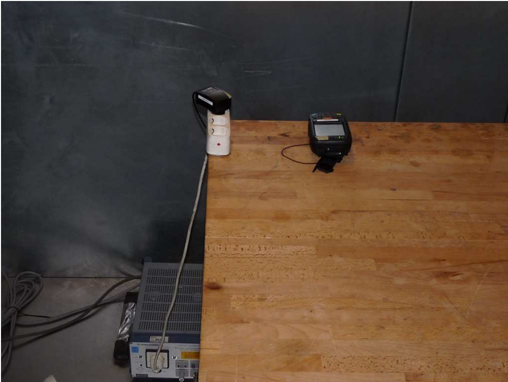
Photo 8: Test setup for conducted measurements (AC Port (power line))
