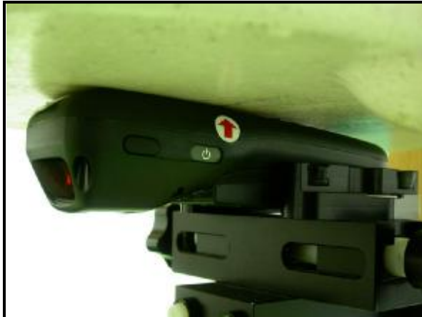
A: The front of the EUT face to the phantom with 0mm-separation distance.
