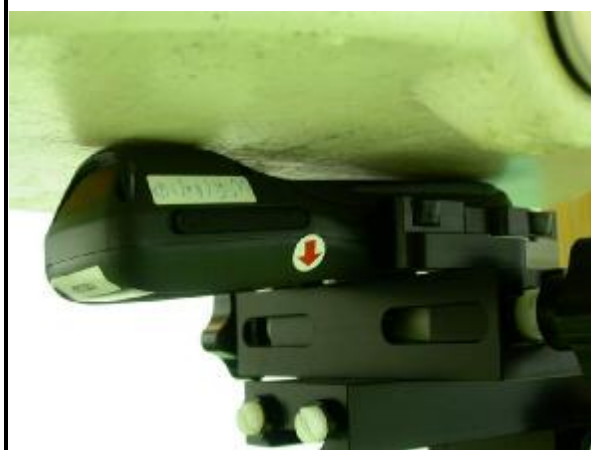
C: The bottom of the EUT face to the phantom with 0mm-separation distance.
