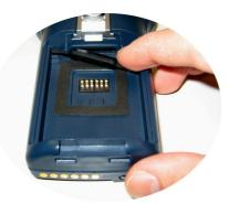
3. Insert the card with the written part upward (as shown in the figure) and push it in, aided by the stylus, until it clicks into place.
