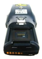
2. Remove the Mini SD card slot's protective rubber cover.
