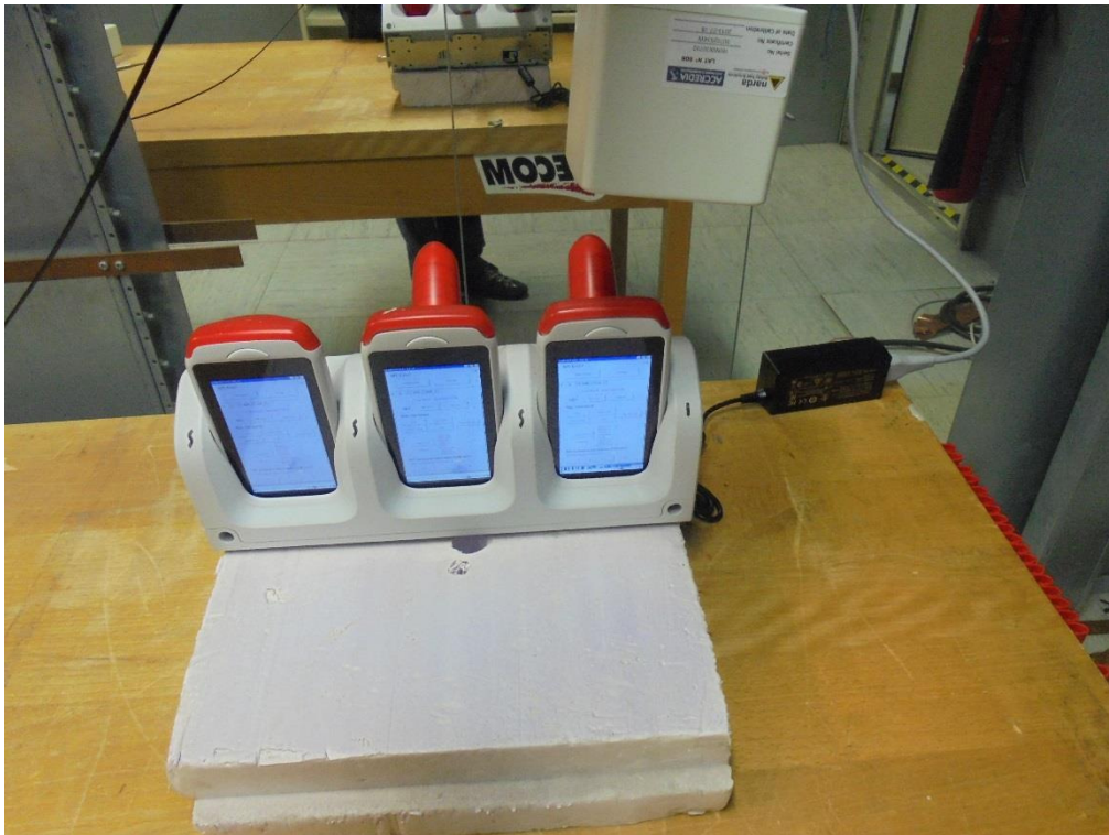
Photograph 3 Measurements in the anechoic chamber, 10cm distance between measurement probe and EUT
