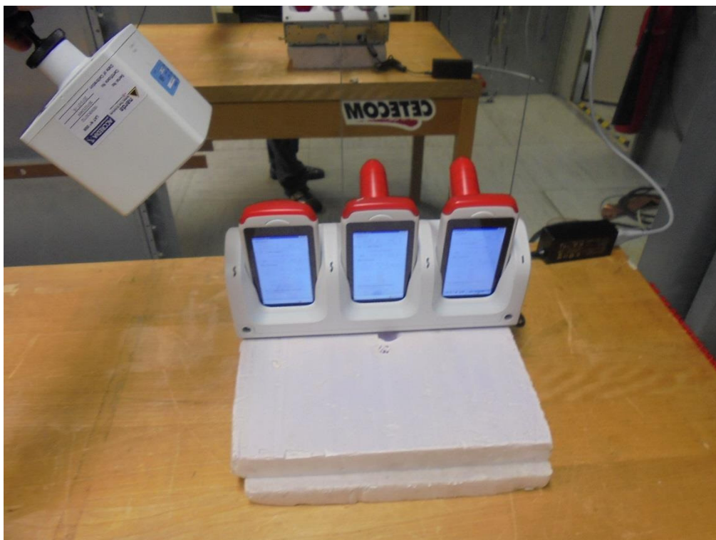
Photograph 2: Measurements in the anechoic chamber, 10cm distance between measurement probe and EUT
