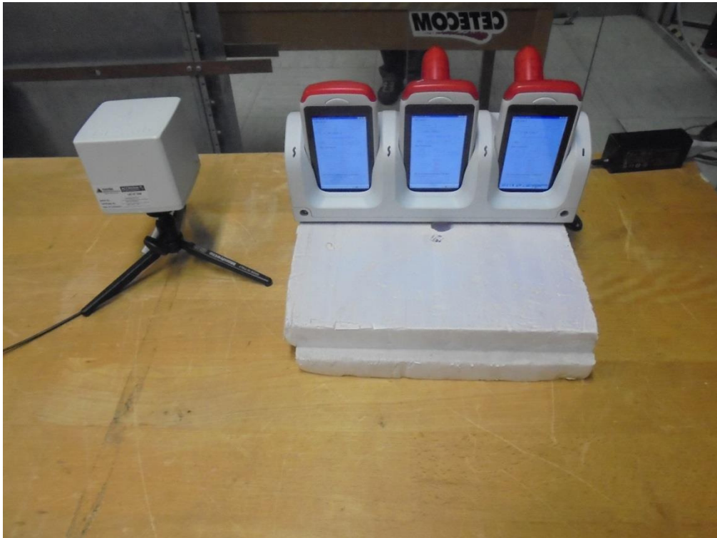
Photograph 1: Measurements in the anechoic chamber, 10cm distance between measurement probe and EUT
