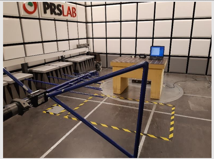
PHOTO N° 3 – SETUP FOR RADIATED EMISSIONS 30MHz – 1GHz
