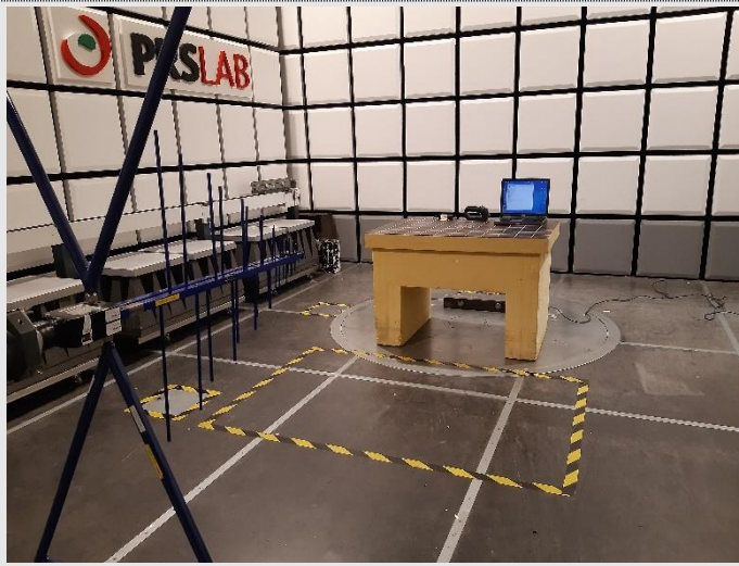
PHOTO N° 3 – SETUP FOR RADIATED EMISSIONS 30MHz – 1GHz
