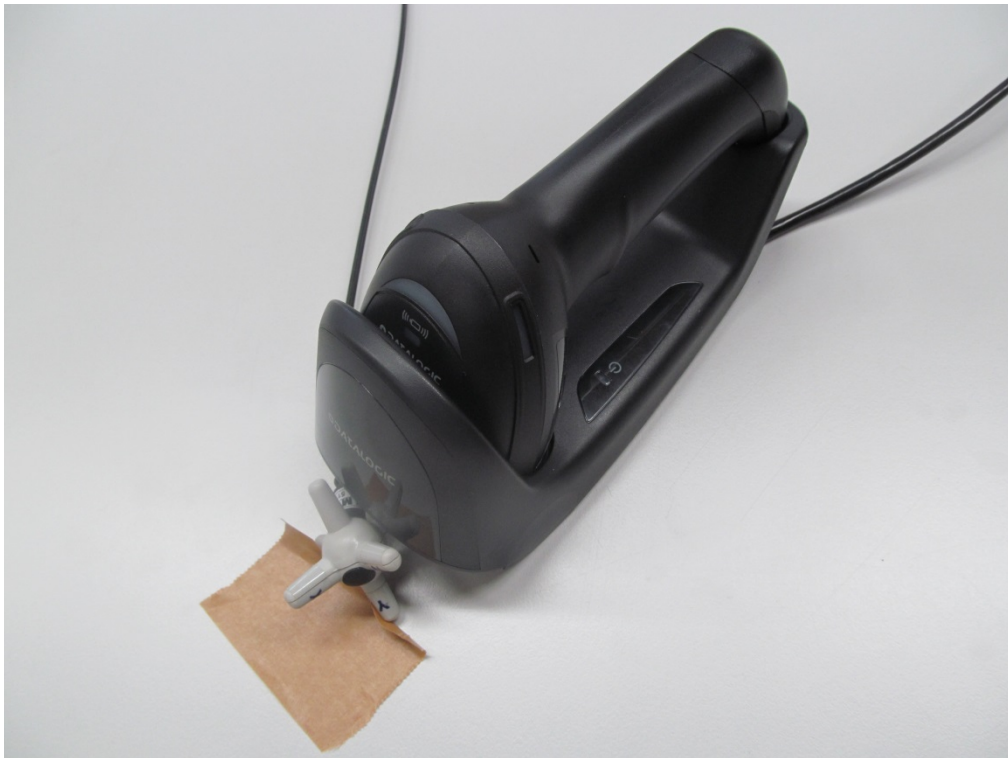
Photograph A1-4: RF H-field strength measurement (distance 0 mm)
