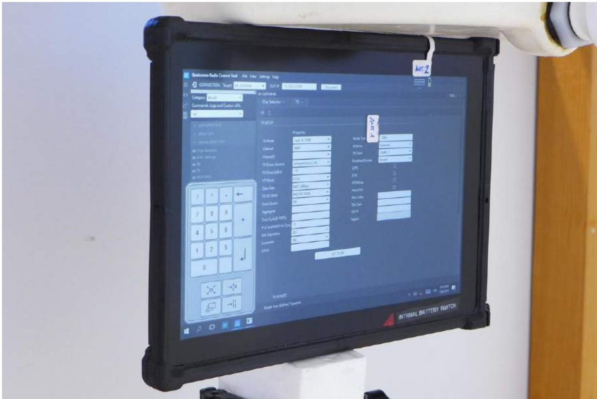
Pic. 4: Test position, edge 4 of DUT towards the phantom, 0 mm distance.
