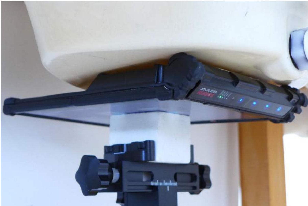
Pic. 3: Test position, back of DUT towards the phantom, 0 mm distance.
