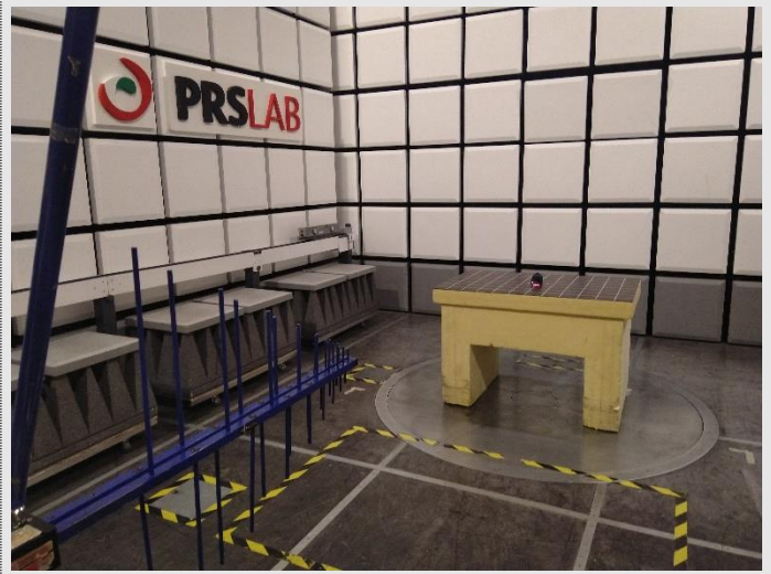
PHOTO N° 2 - RADIATED EMISSION TEST SETUP
