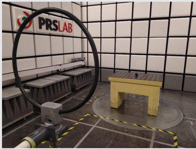
PHOTO N° 2 - RADIATED EMISSION TEST SETUP
