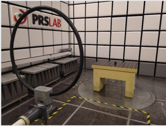
PHOTO N° 2 - RADIATED EMISSION TEST SETUP
