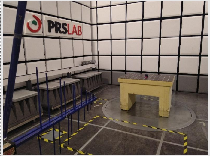
PHOTO N° 2 - RADIATED EMISSION TEST SETUP
