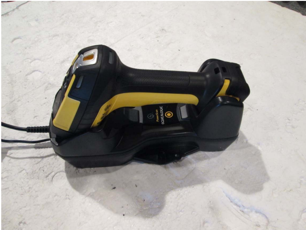
Photograph A1-4: Reader in charging stand EUT #1
