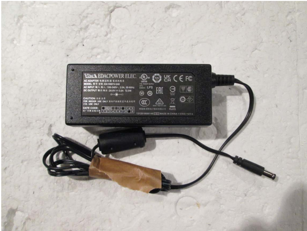
Photograph A3-1: Power supply
