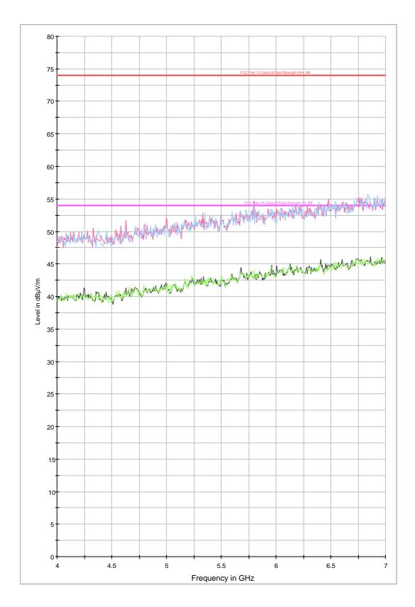
FCC Part 15.109 Radiated Emissions Class B 4-7GHz
