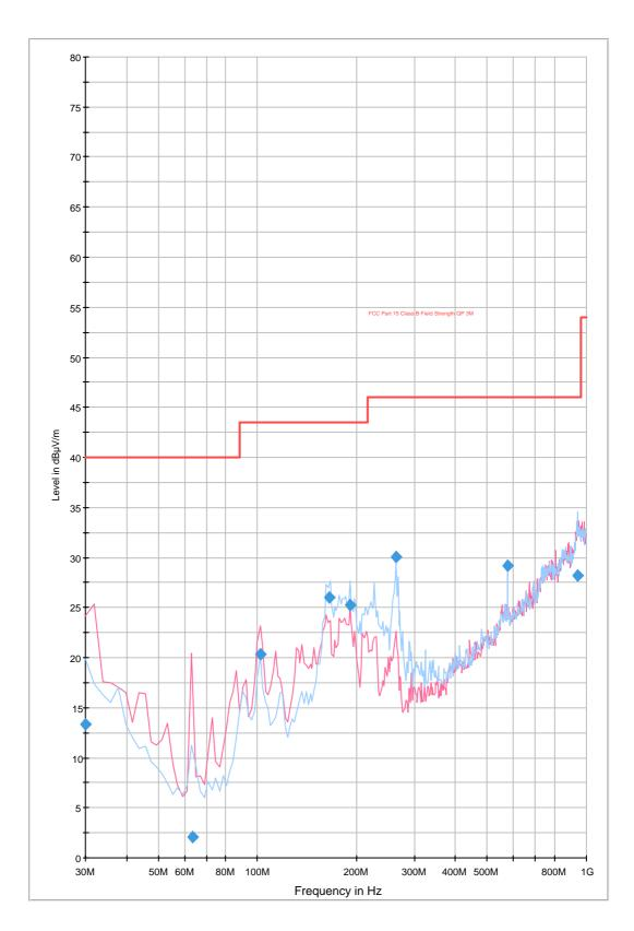
FCC Part 15.109 Radiated Emissions Class B 30MHz-1GHz
