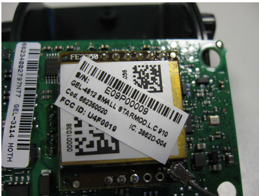
Fig. 6: particular of the label on the radio module
