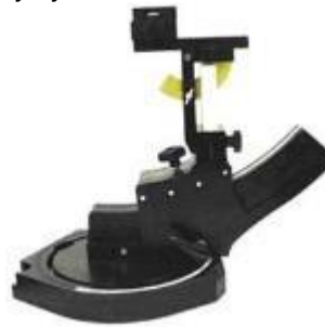
Device holder supplied by SPEAG
