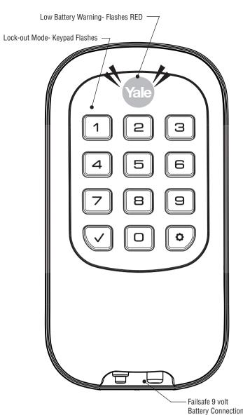
Master PIN Code must be created before any further programming. Max User Codes = 100
