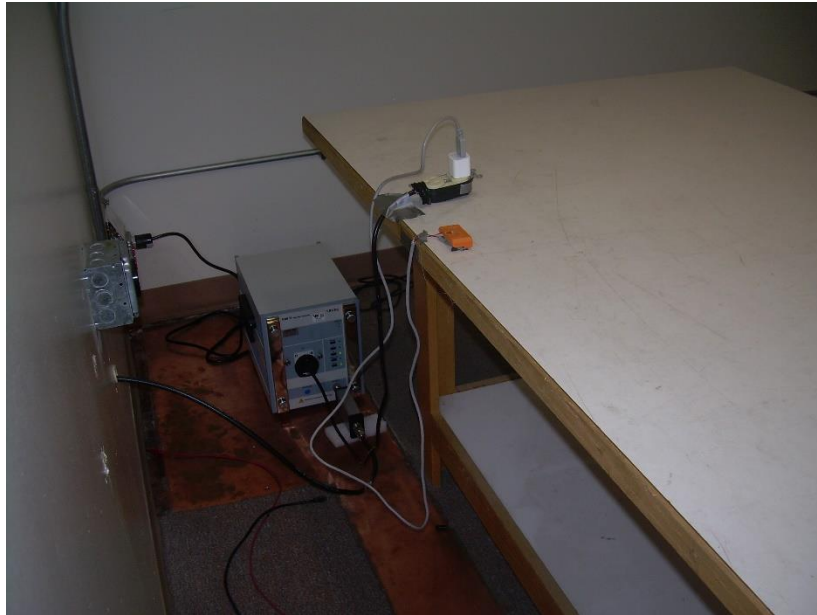
Photograph 9: Back View Conducted Emissions Worst-Case Configuration
