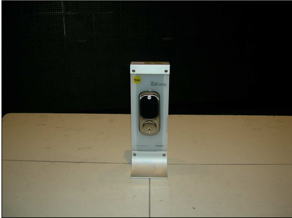
Figure 3: Radiated Emissions – Touch Screen Deadbolt Lock
