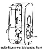
a. Ensure that gasket on inside mounting plate is properly fitted. Note the positioning of the gasket's five rubber nubs (Figure 3A).
