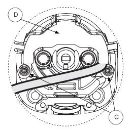
2. Slide new cylinder into sleeve.
